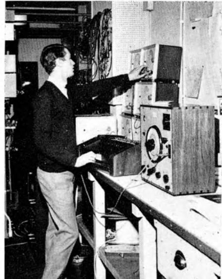
A corner of the BBC Radiophronics Workshop. The audio signal generators are coupled to a keyboard system providing varying degrees of attack and decay.
