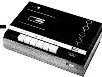
THIS is a well designed set of equipment for the completely non-technical user. The cassette can be changed or turned over with less effort than loading a gramophone record on a turntable. It is stereo all the way, no provision being made for using the four tracks individually. The tracks are recorded in pairs whenever the record key is pressed so that mono record or play is only available by selecting or paralleling the input connections.
