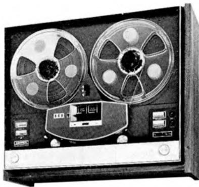
$7\frac{1}{2}$  and  $3\frac{3}{4}$  i/s, frequency response at these speeds being 40Hz-15kHz  $\pm 3$ dB and 50Hz-7.5kHz  $\pm 4$ dB respectively. Unweighted signal-to-noise ratio from peak recording level to broad-band noise is 46dB at  $7\frac{1}{2}$  i/s and 43dB at  $3\frac{3}{4}$  i/s. No equalisation is provided for  $1\frac{1}{2}$  i/s. Playback is to preamplifier stages, the unit being intended for use with external power amplifiers.
