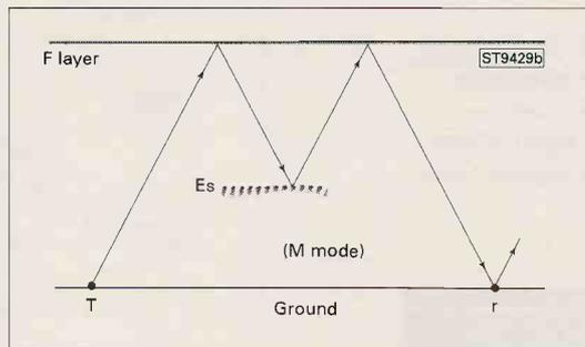
Fig. 2.4: Ionospheric propagation (A) 'N' mode. (B) 'M' mode. Es: Sporadic E cloud (see text).
