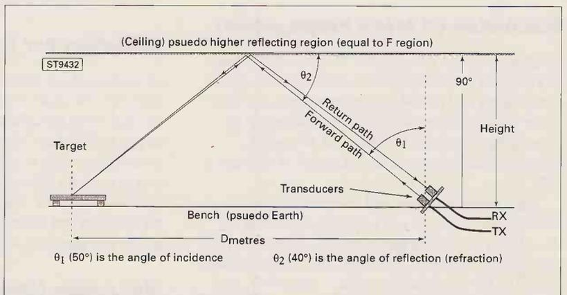
Fig. 2.8: Arrangement for simulation of Over The Horizon Radar (OTHR).
