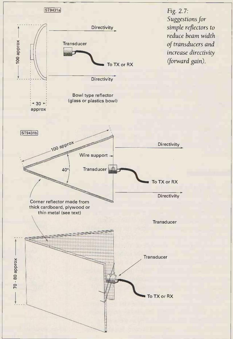
Fig. 2.7: Suggestions for simple reflectors to reduce beam width of transducers and increase directivity (forward gain).
