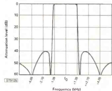
**Fig. 1: Theoretical response of a two-section half-lattice crystal filter.**
