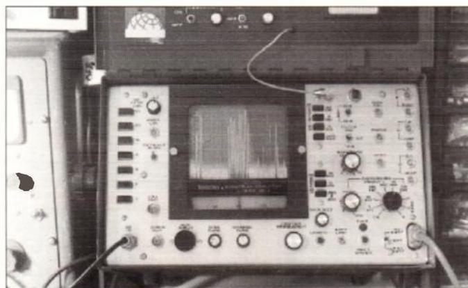
**The Texscan Spectrum Analyser AL-51A displaying the received signals present on a discone antenna between 50 and 150MHz, the central cluster being the v.h.f. f.m. commercial band.**
