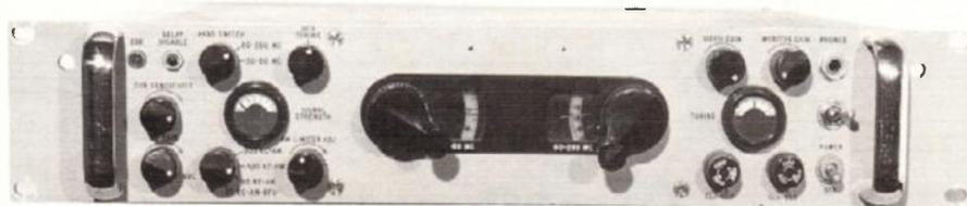
**The Vitro 1907 RX, tuning 30 to 260MHz, a.m./f.m./s.s.b., Signal strength meter to the left, f.m. centre tuning meter to the right, separate tuners and tuning knobs for the two bands.**
