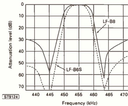
**Fig. 2: Typical low-cost ceramic filter.**
