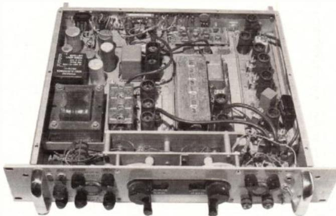
**The Vitro 1907 internal view, 30 to 60MHz tuner to the centre left, 60 to 260MHz tuner to the centre right, i.f. strip along right wall with p.s.u. section on the left.**
