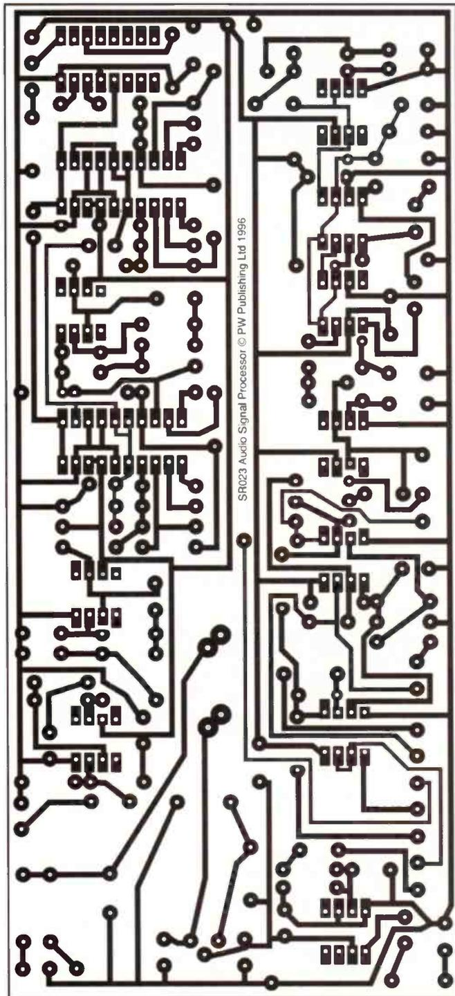
Fig. 2.4: The printed circuit board copper track pattern shown actual size.
