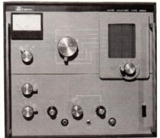
**The Airmec 248A Wave Analyser, tuning 5 to 300MHz in six bands, a.m./f.m., With large 'S' meter top left, input socket lower right.**
