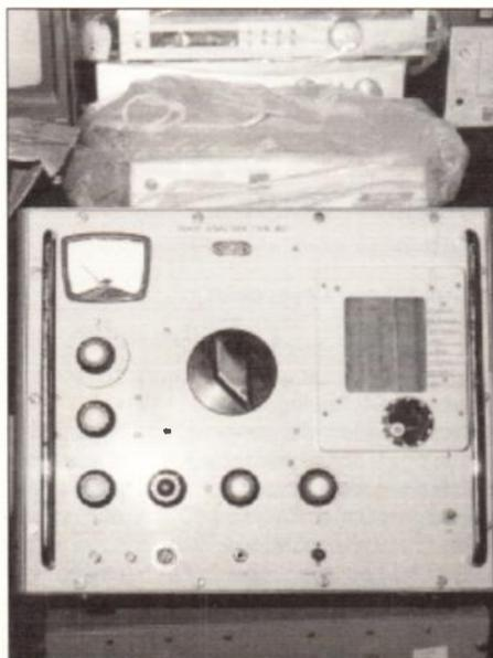
**Another Airmec 'receiver', this is the Type 853, tuning the h.f. frequencies though, 30kHz to 30MHz.**
