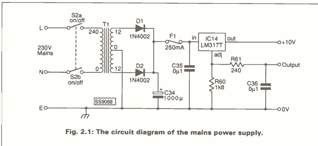
Fig. 2.1: The circuit diagram of the mains power supply.
