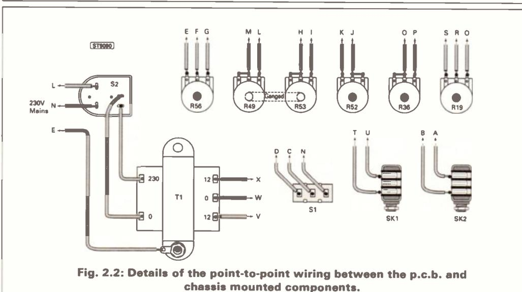
Fig. 2.2: Details of the point-to-point wiring between the p.c.b. and chassis mounted components.
