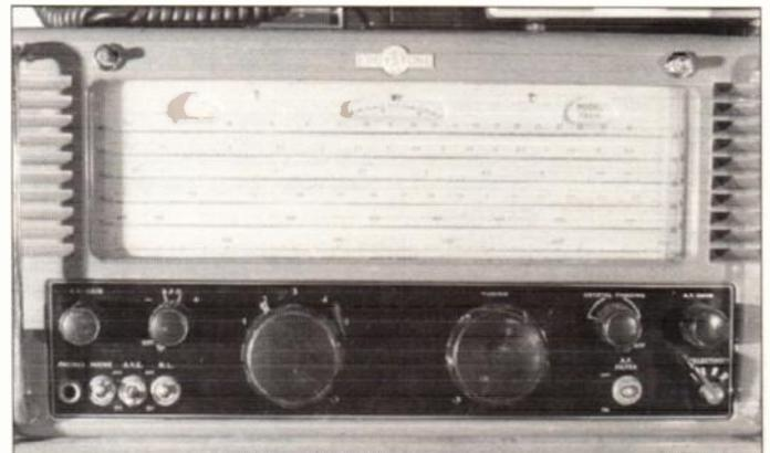
**The familiar Eddystone layout with its large, easy to read, dial scale. Whilst this set is the 730/4 h.f. set, the layout is identical to the 770 series v.h.f. and u.h.f. receivers.**
