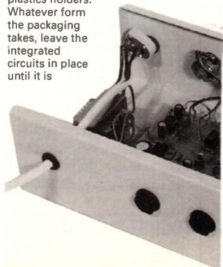
time to fit them onto the board. They must be fitted into d.i.l. holders, and not soldered directly onto the board. Do not fit them into their holders until the board and all the wiring has been completed.
