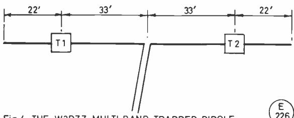
Fig.4 THE W3DZZ MULTI-BAND TRAPPED DIPOLE.
