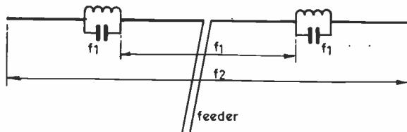
Fig. 1a A TWO-BAND TRAPPED DIPOLE
