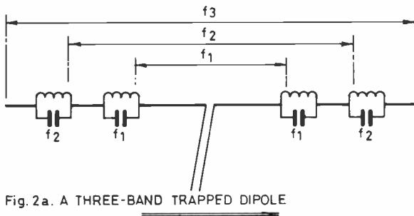
Fig. 2a. A THREE-BAND TRAPPED DIPOLE
