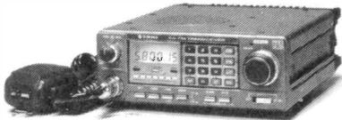
**TS930S HF TRANSCEIVER WITH GENERAL COVERAGE RECEIVE FACILITIES**
