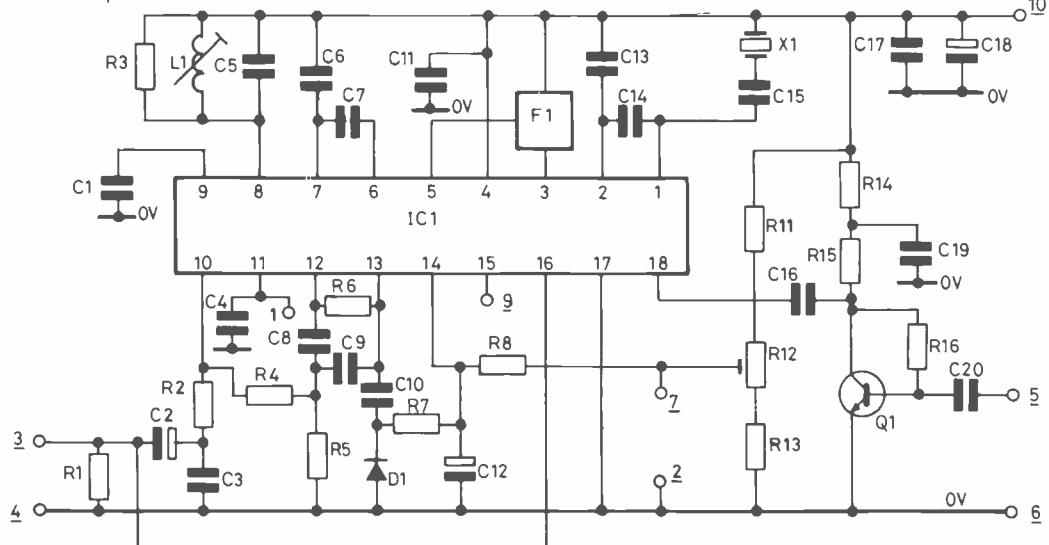
**Fig. 2 FM707 DEMODULATOR CIRCUIT**
