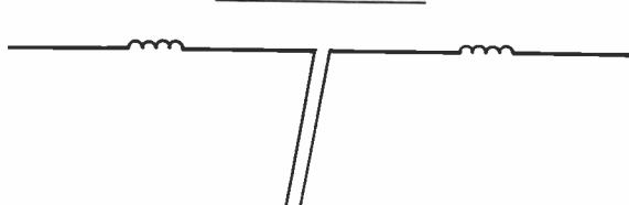
Fig. 1c. EQUIVALENT CIRCUIT OF THE TWO-BAND TRAPPED DIPOLE WHEN OPERATED AT FREQUENCY  $f_2$
