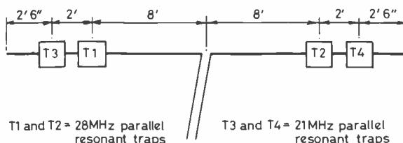
Fig. 7 TRI-BAND TRAPPED DIPOLE FOR 14/21/28MHz.
