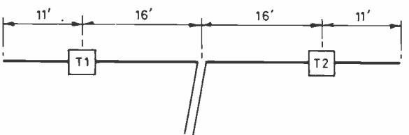
Fig.5 FOUR-BAND TRAPPED DIPOLE FOR 7, 14, 21 & 28MHz.
