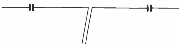
Fig. 3 EQUIVALENT CIRCUIT OF A TWO-BAND TRAPPED DIPOLE WHEN OPERATED ON A FREQUENCY HIGHER THAN THE RESONANT FREQUENCY OF ITS TRAPS.
