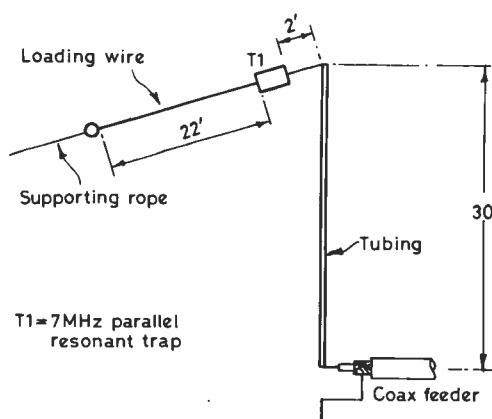
Fig.11 A 5-BAND INVERTED-L
