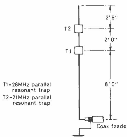
Fig. 9 TRAPPED VERTICAL FOR 14/21/28 MHz
