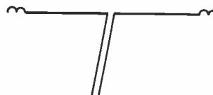
Fig. 1b. EQUIVALENT CIRCUIT OF THE TWO-BAND TRAPPED DIPOLE WHEN OPERATED AT FREQUENCY  $f_1$
