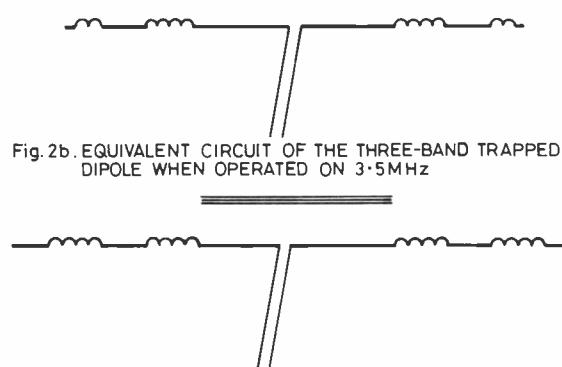
Fig. 2b. EQUIVALENT CIRCUIT OF THE THREE-BAND TRAPPED DIPOLE WHEN OPERATED ON 3.5 MHz
