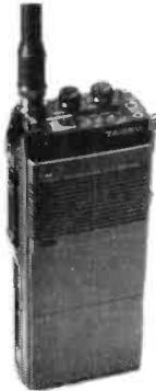
The ultra compactness of the FT203R is due mainly to Yaesu's chip component circuit board assembly, the chip components being installed automatically by robots. The 203's features include thumbwheel frequency selection, built in S/PO meter, 2.5W RF O/P at 10.8V, (3.5W O/P with FNB4). Vox activated switching is possible when used in conjunction with YH-2. Accessories supplied include FNB3, FTE-2 tone unit, CSC6 case and YHA-14A antenna.
