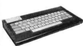
This microprocessor-based product is the ultimate in 'electronic keyers' and will send both live and stored messages in the speed range 12–30 wpm.
