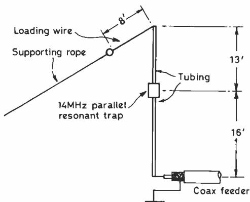
Fig.10 THE "XAP 2V" INVERTED-L FOR 14/21MHz
