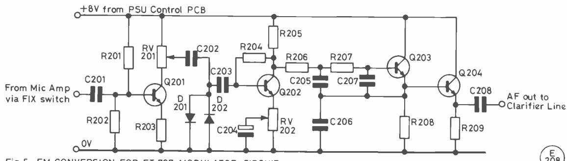
Fig. 5 FM CONVERSION FOR FT-707 MODULATOR CIRCUIT
