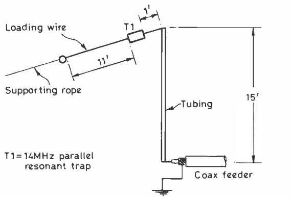
Fig. 12 A 4-BAND INVERTED-L
