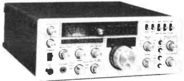
FT-107M. This is the brand-new solid-state HF Transceiver which has just been included in the ever-growing range. The receiver performance is comparable to the FT-901 (which says everything) and a memory option is provided of 12 programmable channels plus fine tuning. Add to this the ease of tuning, 240 PEP input, superb low-profile styling and here is the rig for the Eighties.
