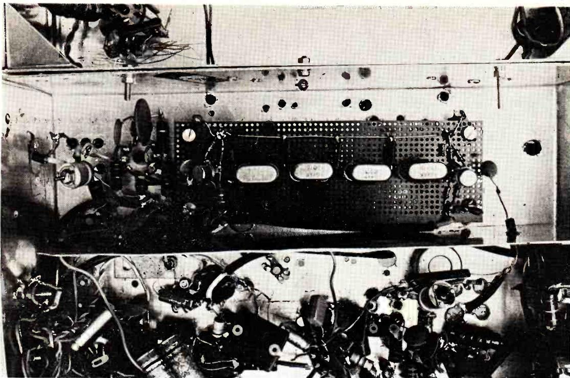
Layout of ladder filter and filter amplifier. The carrier balancing pot and trimmer can also be seen to the left of, and just above, the filter.
