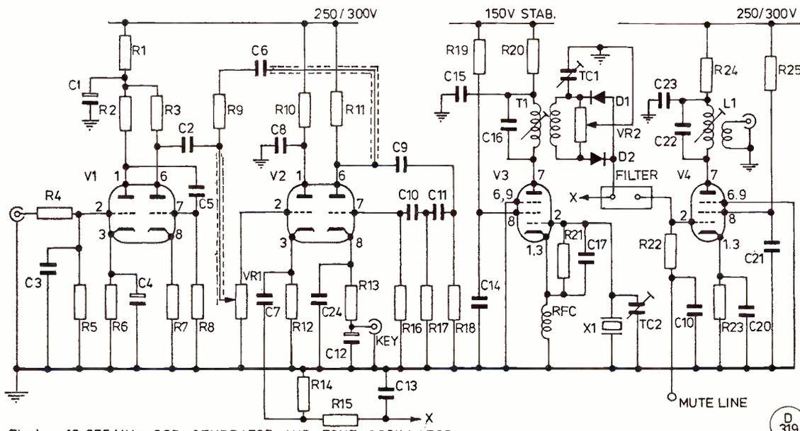
Fig. 1 10.075 MHz SSB GENERATOR AND TONE OSCILLATOR
