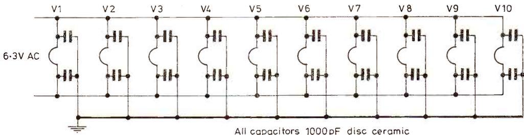
Fig 4 HEATER WIRING
