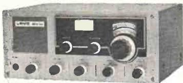
The SRX30 is designed as a budget priced receiver that outperforms many receivers costing 3 times as much. Featuring the Barlow Wadley loop, it will enable you to explore the exciting world of short wave radio—amateurs, broadcast, aircraft, shipping, etc. This is a completely self-contained package, having all the features necessary for complete and reliable coverage of the frequency range 0.5 MHz to 30 MHz.
