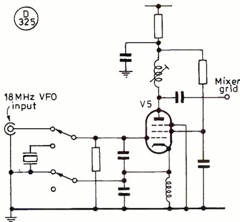
Fig. 5 One method of switching the EF80 conversion oscillator to buffer mode
