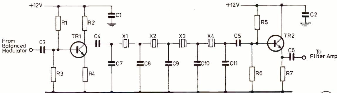
Fig. 1a 10.075 MHz LADDER FILTER AND MATCHING CIRCUITRY
