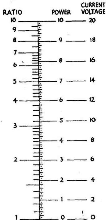
Values of dB corresponding to power ratios from 1-10 can be obtained from this scale.
