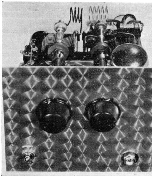
Coils for five metre reception are as follows:—L1, four turns of 16 S.W.G. enamelled copper wire wound on a ¼-inch former, the ends being used for support from the aerial condenser. This coil is home-constructed, for a commercial coil with a base cannot be adjusted to the correct coupling. L2 is a commercial 5-turn coil; or, for those desiring to make their own, 5 turns of 16 gauge wire.
