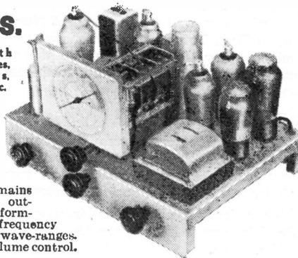
De luxe all-mains chassis with outstanding performance. Radio frequency amplifier. 3 wave-ranges. Automatic volume control.
