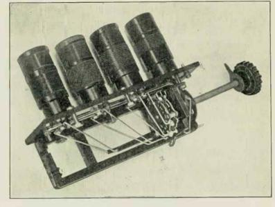
Side view of short-wave coil shelf, and double-pole switch with its extension handle.
