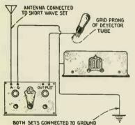
Fig. 8. How aerial and ground are connected to set and converier.
