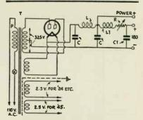
Wiring diagrams of the HY-7B plate, filament and heater supply.
