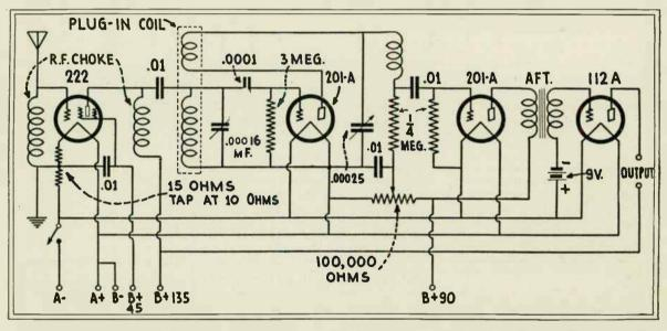
Fig. 4 above shows connection of a 222 tube in the RF circuit ahead of the detector, with detector feeding into a resistancecoupled stage of audio frequency amplification. The use of a screen grid tube eliminates dead spots on the tuning dial.
