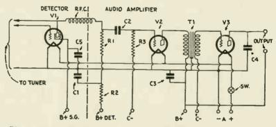
Diagram above shows Mr. Barnett's favorite audio amplifier hook-up for use in short-wave reception. Note that resistance coupling is used in the first audio stage to prevent "fringe howl".
