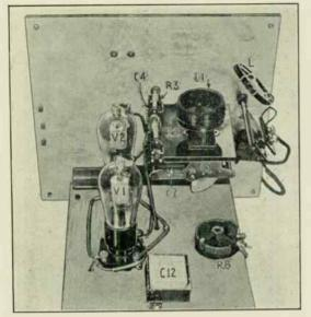
Fig. 2-Close-up of first R.F. stage in Mr. Marshall's S.W. receiver.
