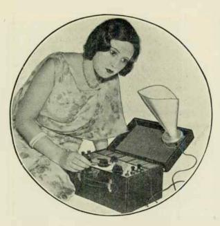
The "S.W.C." specially designed "short wave" portable in operation in the Editor's office. Works loud speaker on two tubes, battery operated, no plug-in coils, light in weight, and other features.
