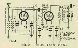
whose average diameter is 1% inches; they are of truly skeleton construction and, if wound with 27/42 D.S.C. Litzendraht wire, will be found to be extremely efficient. For C1 and the tank capacity C2, the Hammarlund "MC/23" condensers can be used as very little surplus metal appears in their construction. The vernier, which is wired in parallel with C2, is an "R.E.L." adjustable, but Cardwell's new type will serve just as well.
