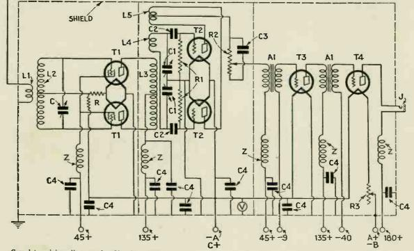
Complete wiring diagram for Mr. Schnell's exceptionally efficient and selective short-wave receiver, in which he employs push-pull action for the radio frequency as well as the detector stages. The audio section comprises two stages of transformer coupled amplification.
