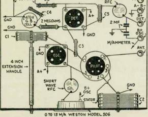
Top view of One-Coil Super-Het S-W Converter.
