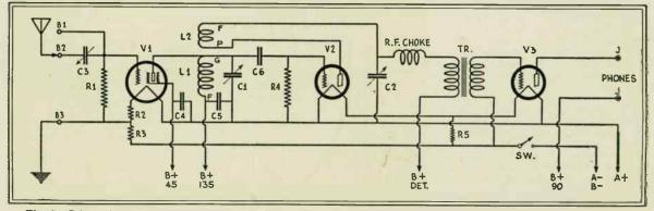
Fig. 1. Scher "Craft Box." Schematic circuit to be followed by those who want to dig into their junk box and ride the short waves via the Box." As 90% of construction is getting started, "it's up to you"; we have eliminated all the mechanical difficulties.
