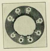
Fig. 6, above, shows the jack arrangement of eight connections, three for the plate inductance screen-grid tubes, two for the secondary, and three for the tickler.
