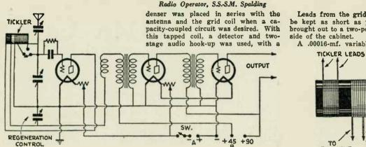
Leads from the grid inductance must be kept as short as possible, and are brought out to a two-point switch on the
