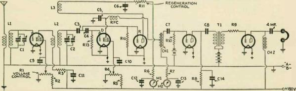
Complete hook-up of the Somerset short wave receiver, with separate reactor tube "R," used solely to provide smooth and reliable regeneration control. The regeneration is regulated by the variable resistance R11. Detector tube "D," is impedance-coupled to the first audio stage.
