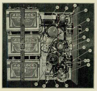
Fig. C. Batteries in place; all leads connected; tubes in their places.
