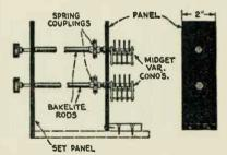
Preferred manner of mounting the midget variable condensers, which are controlled by bakelite extension rods and knobs.
