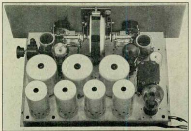
Rear view of the HY-7B super-het, showing shielded coils and tubes.
