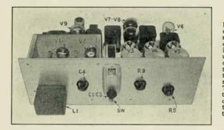
Fig. A In this front view of the "SWS-9," the single plug-in inductance L1 is seen in its shield. This unit contains both oscillator and antenna coils, the details of which are shown in Fig. 4. The power pack, at the left, rear, introduces no perceptible hum. This set tunes with superb ease.
