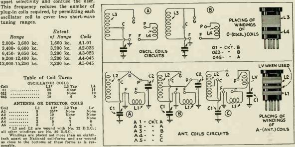
Details of oscillator and antenna coil circuits.
