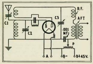
Fig. 2 above shows how to smooth up the regeneration con-trol on short wave receivers—use a potentiometer at "P," to give fine control of the plate voltage.
