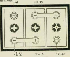
Diagram above shows how the author provides "A" current at 2 volts, also "C" voltages of 2 and 4 volts from standard, six-volt storage battery.
