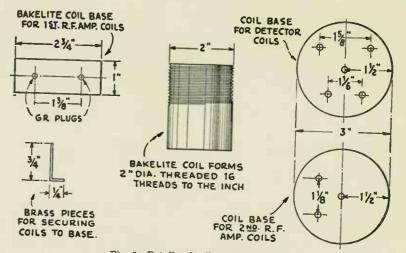
Fig. 6-Details of coils and coil bases.
