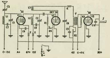
The usual method for controlling filament voltage is with a fixed resistor and a variable rheostat for critical adjustment, but without a voltmeter this is purely guesswork. To overcome this difficulty, and gain an advantage, the method of using a single storage cell has been adopted; this eliminates the use of all rheostats and resistors.
