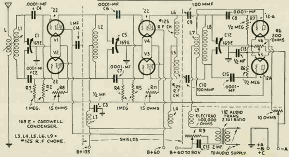
Fig. 1-Wiring diagram for Mr. Marshall's receiver, utilizing two push-pull R.F. stages, feeding into a push-pull detector stage, providing superior sensitivity and selectivity in short-wave reception.
