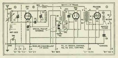
Fig. 3—The Superregenode circuit for battery operation; see Fig. 11 for the detail of the "whistle filter." A push-pull output transformer for '45s is a good match for the '33 pentode.
