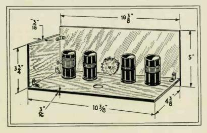
Tuning and control panel of portable short wave set.
