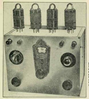
A NYONE can assemble this simple self-contained short-wave receiver in United States and foreign stations throughout the world. It is a onetube, complete with batteries installed in the 10 x 8 x 6 inch aluminum radio shield can. You can pack it into a grip or carrying case and carry it wherever you go. After having acquired skill in the manipulation of the set with earphones, you can attach it with one wire
