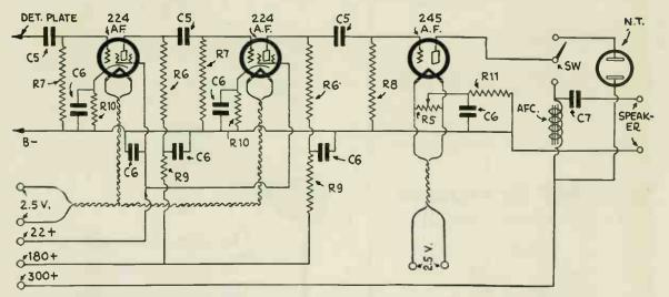
Fig. 2-Circuit of television audio amplifier with filters to prevent motor-boating, and switch to change from pictures to voice.
