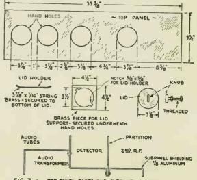
FIG. 7 - TOP PANEL ,PARTS AND SUBPANEL SHIELDING.
