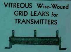
Unique construction allows for winding more wire of a larger diameter in small space. Liberally insulated. Soldering lugs and contact bands of Monel metal, assuring equal expansion and positive connections. Vitreous enameled. Guaranteed not to develop noise or open circuits.
