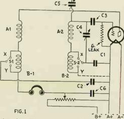
MIDGET (2-S PLATE) .0002-MF. Assemble the four Pilot four-prong No. 214 sockets in the holes provided; arranging them so that the "G" and "P" terminals are G. LEAK Ś Gd 00 .01-MF. toward the front end of the sy panel or shelf. Two 1/2-inch 6-32 R.H. machine-screws are placed in the two holes at the very front edge of .01-MF. RESISTOR SWITCH 1 ME 0 a Fig. 5-Wiring external to the short-wave coil panel is ٦ B+"
