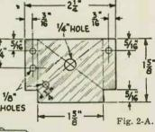
Fig. 2-A — Switch support member of insulating material.
