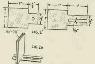
How to make a very small capacity condenser suitable for connecting in series with the antenna for short-wave reception. The two condenser plates are made out of copper, but brass or other non-magnetic metal will do.
