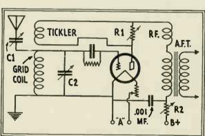
Fig. 3 shows still another way of controlling regeneration by varying the plate potential on the detector tube with a finely variable resistance R-2; and also by the variable resistor R-1.
