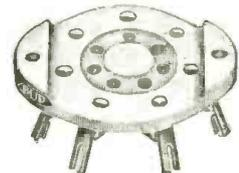
Circuits requiring very low loss construction will find this line of Glazed White Ceramic Sockets the perfect receptacles for tubes and plug-in coils. The contact springs are of a special design that assures a positive contact indefinitely on a large area of the pins, and these springs have heavy soldering terminals. Priced only 24c to 33c net at your BUD jobbers.
