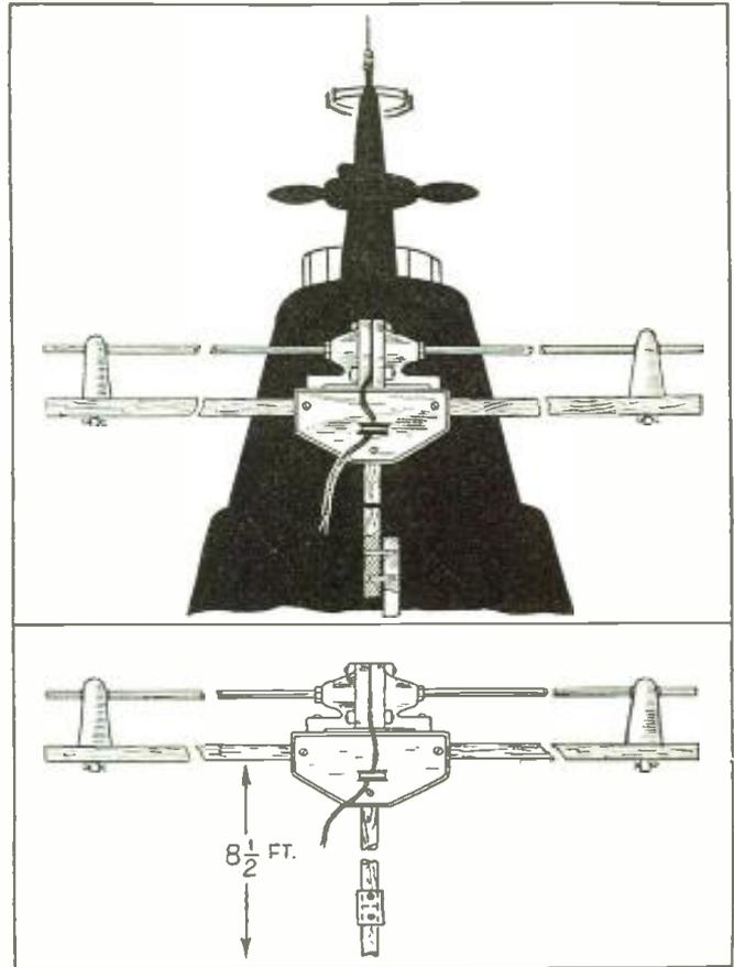
▲ Above, top, the antenna is erected perpendicular to the beam from the transmitter. Detail of antenna construction appears in the panel.
