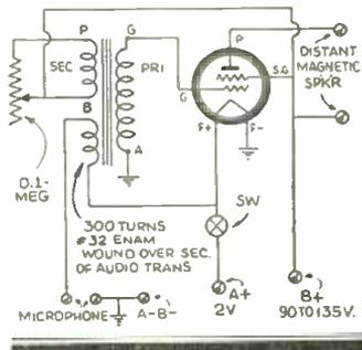
135 volts of "B" battery. The microphone is of the single-button carbon type.—*Paul F. Hatten*.
