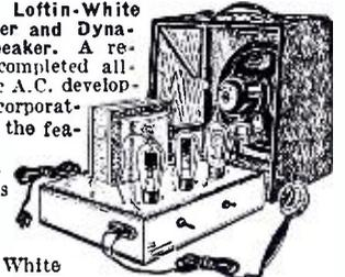
Loftin-White Amplifier principle. The amplifier is a high quality two stage job, having some RADICALLY NEW IDEAS IN AUDIO FREQUENCY AMPLIFICATION and employing 1-27, 1-45 power tube and 1-80 full-wave rectifier. It is remarkably free from A.C. hum.
