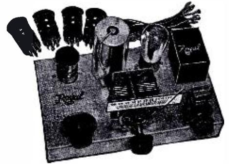
Note the neat construction of the Royal S-W receivers: plug-in coils in background.
