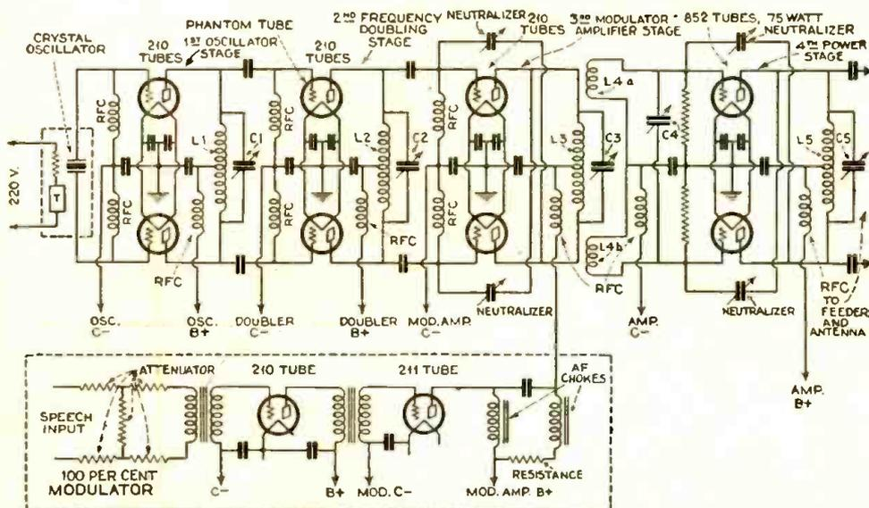
Fig. 1. Complete circuit diagram for the push-pull short wave transmitter with crystal control and frequency doubler circuit, as well as 100 per cent modulator circuit.
