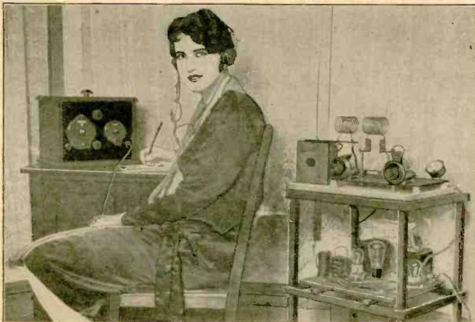
used. The receiving set used by Miss Peiser is shown at the left of the picture. High ratio vernier dials are used on the receiver to enable the operator to do very fine tuning. Miss Peiser has taken a great interest in amateur radio communication—and by the way, this is a mighty fine way to get acquainted. We have read of many courtships which started "via the ether". So girls, here's your chance to get acquainted with many he-males — become a short-wave fan!
