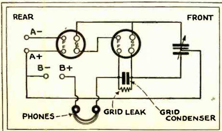
The diagram at the left shows connection of balanced variable condenser, together with grid condenser, grid-leak and phones, and V-T sockets; the socket at the extreme left being used for the tube and the one at the right for the inductance, which is fitted with an old tube base or its equivalent.
