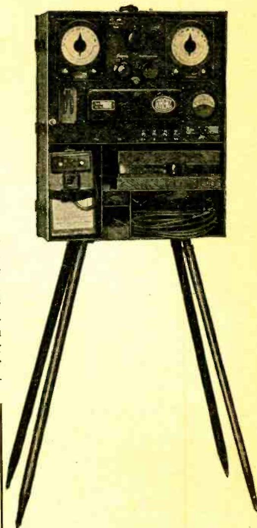
Fig. 17. Short-wave radio receiver, built in two compartments, by the famous Lorenz concern of Germany. This set works with the transmitter shown in Fig. 13.
