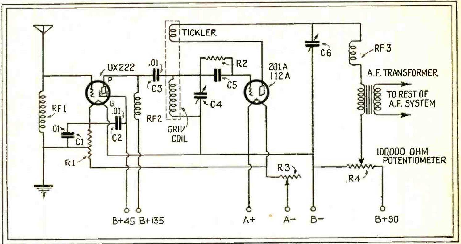
Fig. 3. The circuit above shows how to connect a 222 tube in an RF stage ahead of the regenerative detector; this simple addition to your old short wave set gives far greater stability and evenness of tuning.
