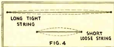
Fig. 4. This diagram shows how musical vibrations are set up by a long, tight string, on the piano for example, while a short, loose string does not give what we would call musical vibrations, but will merely flop about without really vibrating.
