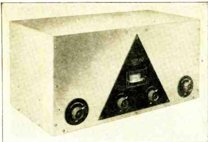
Front view of Norden-Hauck de Luxe short-wave receiver, known as the Super DX-5. It measures 9" by 18" by 10" and weighs 30 lbs. Wavelength range 20 to 205 meters and adaptable down to 10 meters, and as high as 2000 meters with extra coils.
