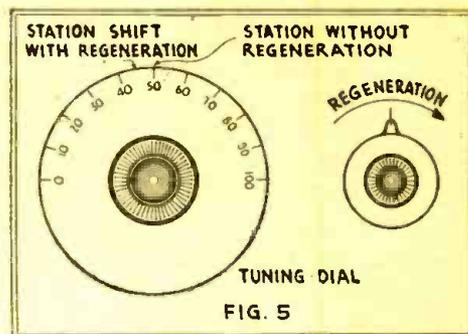
Fig. 5. This diagram shows how, in tuning a short-wave set, one has to "follow the station" on the tuning condenser dial, as regeneration is changed to strengthen the signal. In other words, the change in the regeneration changes the tuning.
