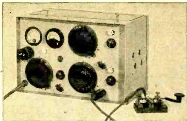
Fig. 2. This photograph shows the appearance of a German-built, 2 watt, short wave transmitter, this particular transmitter with operating key shown at right of the picture being the one used on the famous dirigible "Graf Zeppelin". The dials for tuning the condensers in the short wave transmitter are the usual type and necessary milliameters are incorporated on the panel, together with filament resistance controls, etc.
