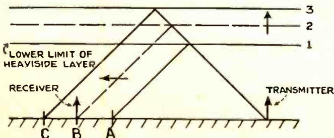
Fig. 4 shows the action taking place in the transmission of a short wave, the wave rising from the transmitter aerial striking the Heaviside layer and being reflected downward.
