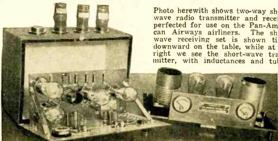
Photo herewith shows two-way short-wave radio transmitter and receiver perfected for use on the Pan-American Airways airliners. The short-wave receiving set is shown tilted downward on the table, while at the right we see the short-wave transmitter, with inductances and tubes.
