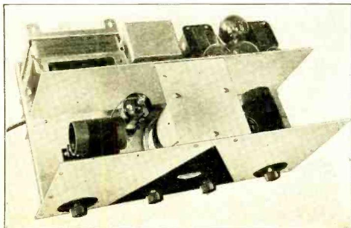
Interior view of Super DX-5 receiver, taken from the top, showing good design and arrangement of the parts. Power pack and audio amplifier are mounted in the rear and suitable shielding used wherever found necessary.
