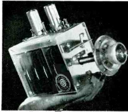
Hoffman silver-circle tuner utilizing printed circuits. Features continuous tuning via a tuning shaft mounted on roller bearings. On the shaft are eight shorting bars that vary the inductance on a printed circuit. There are also eight printed circuits, each photo-etched with silver on insulating material. Tuner has sixteen moving parts that wear eight sliding silver contacts and eight heavy silver tuning lines; eight solid bearings on shaft with one planetary drive and eight bearing surfaces.
