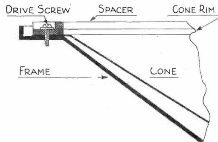
Fold the spacers again to make them "L" shaped, so that they can be placed in the armature gap without falling in. The paper spacers must be placed approximately 120 degrees apart.
