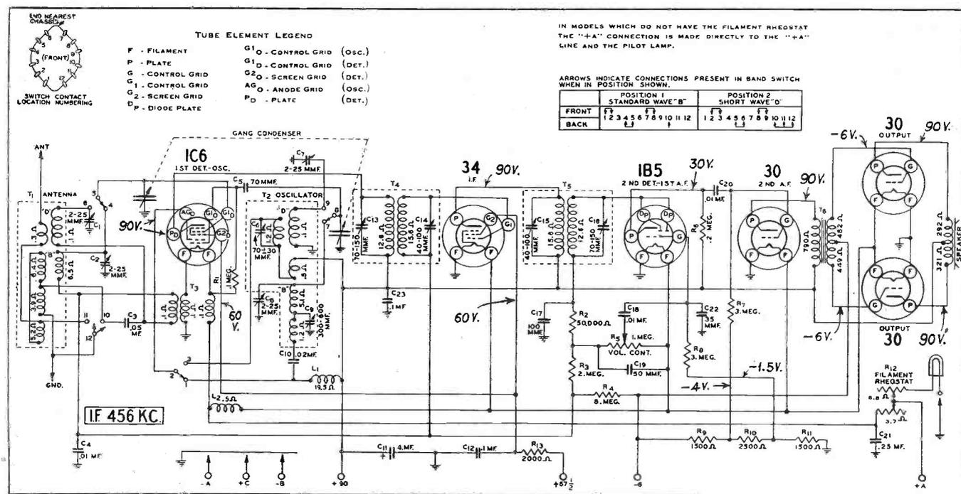
Fig. 1. Wells Gardner 6G circuit diagram.
