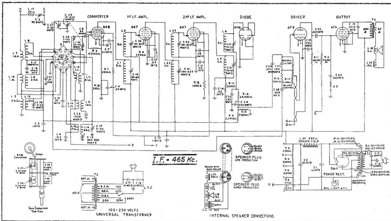
Fig. 1. General Electric E-71, E-72 and E-76 circuit diagram.
