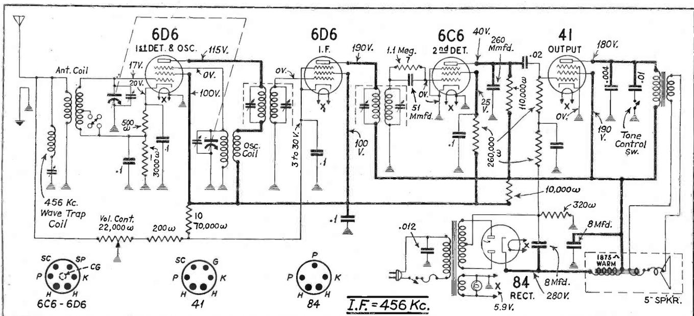
Fig. 1. Stewart Warner R-144AS circuit diagrams.
