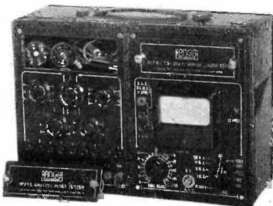
Model 640—Free Point Tester has five (5) sockets. Panel includes automatic switch type and single action jacks.
