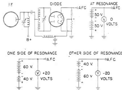
Fig. 6. The a-fc discriminator circuit.
