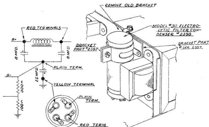
Motorola 50 electrolytic mounting and circuit.
