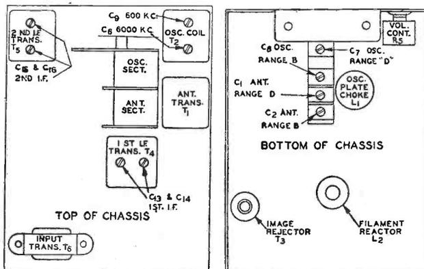
Fig. 2. Chassis views showing trimmer locations.
