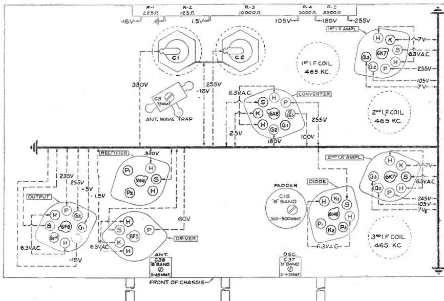
Fig. 2. G. E. E-71, E-72 and E-76 tube and trimmer locations.
