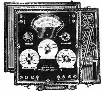
measuring both a-c and d-c microamperes, milliamperes and amperes. Six ranges each are available indicating from 10 microamperes to 2.5 amperes in both a-c and d-c.
