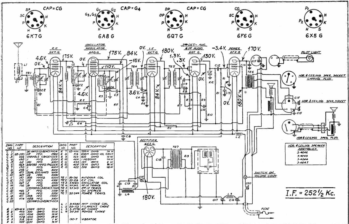
Fig. 1. Zenith 6-M-92 circuit diagram.
