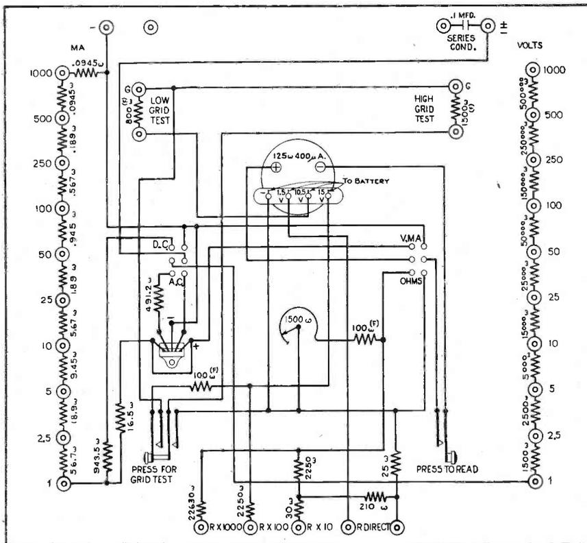
Fig. 1. Weston 665 Analyzer circuit.
