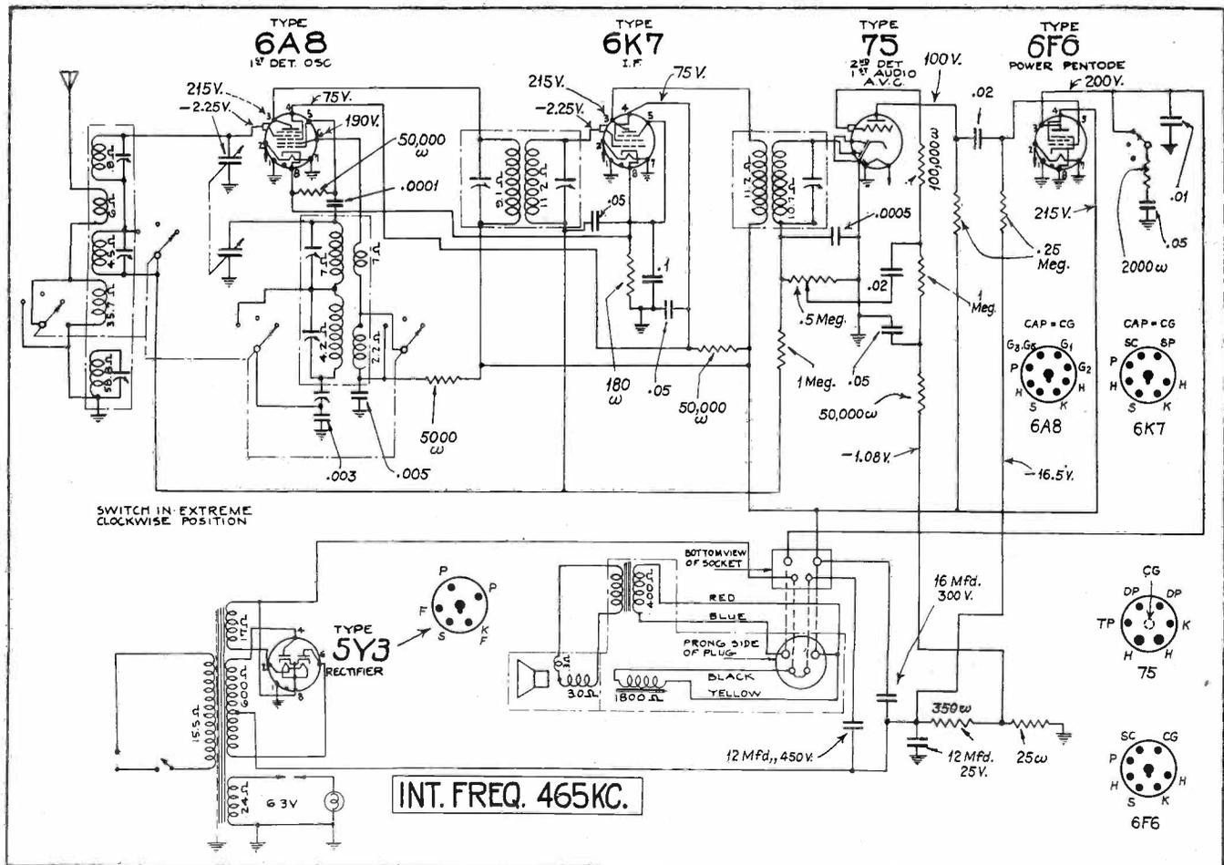
Fig. 1. Bosch 605-605C circuit diagram.
