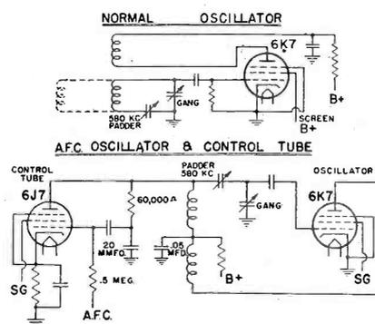
Fig. 4. The afc oscillator circuit.
