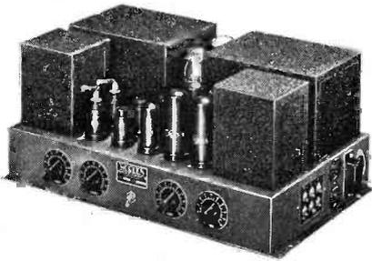
MC120 amplifiers using the 6L6 beam-power tubes.
