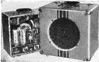
microphone and desk stand housed in a modern luggage case which forms the baffle for the speaker during operation. The C-45 is manufactured by the Transformer Corporation of America, 69 Wooster St., New York City.
