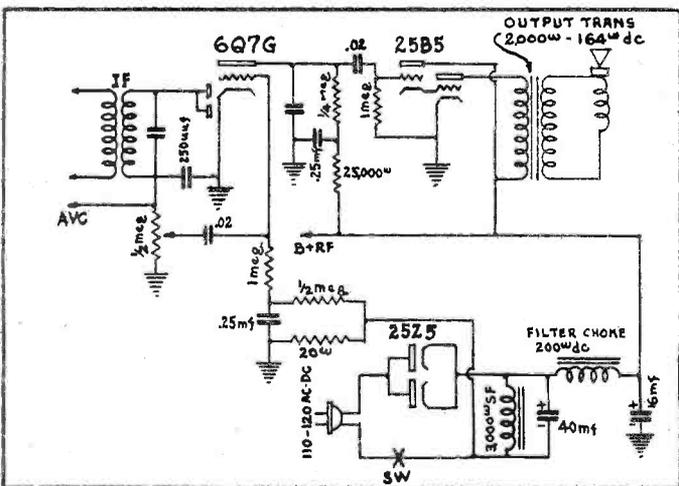
Fig. 6. Schematic diagram of audio amplifier and power supply of set "C" converted for 25B5.
