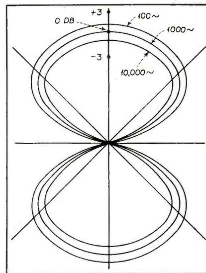
Fig. 2. Directional characteristic of velocity microphone.
