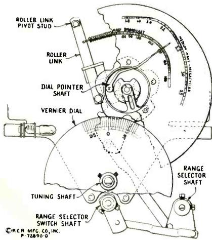
Fig. 2. RCA tuning mechanism.
