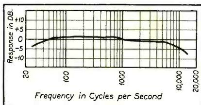
Fig. 1. Response characteristic of velocity microphone.
