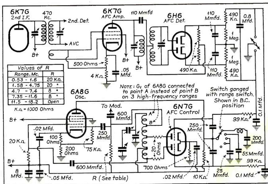
Fig. 2. Philco magnetic tuning circuit.
