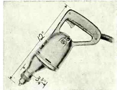
universal motor for d-c or a-c, 25 to 60 cycle operation.
