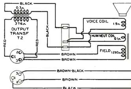
Fig. 4. RCA speaker connections.
