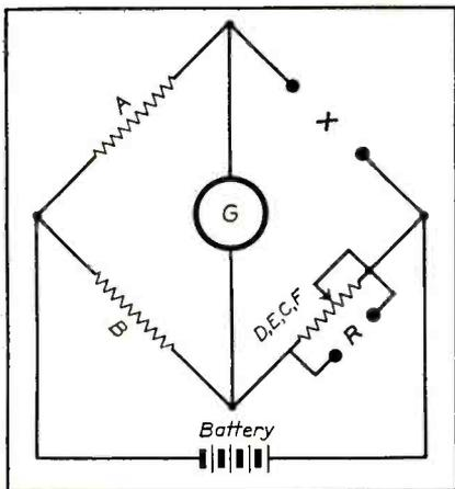
Fig. 1. Fundamental bridge circuit.
