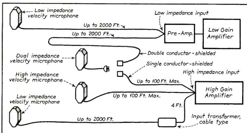
Fig. 5. Velocity microphone connections.
