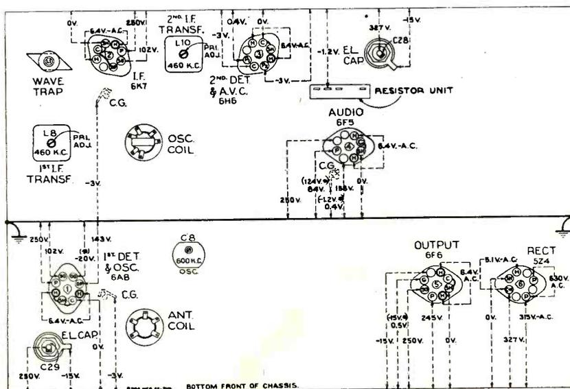
Fig. 2. Socket voltages and trimmer locations.
