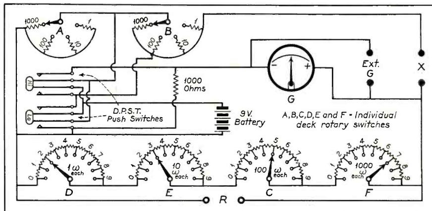
Fig. 2. Wheatstone bridge circuit.
