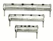
Hi+Q Ceramic Capacitors are of titanium dioxide (for temperature compensating types) and are tested for physical dimensions, temperature co-efficient, power factor and dielectric strength. CI type with axial leads; CN type with parallel leads.
