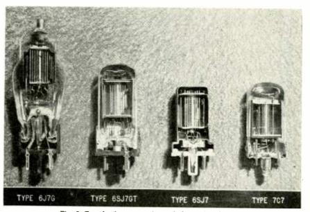
Fig. 6. Four basic constructions of electronic tubes. (Courtesy Sylvania Elec. Co.)
