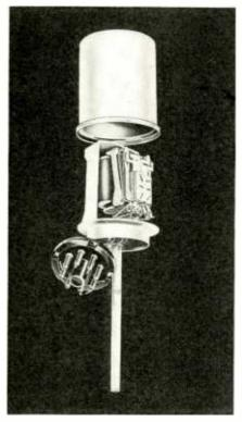
Fig. 9. Sealed relay. Air is exhausted from housing, which is filled with dry nitrogen. (Courtesy Automatic Elec. Co.)
