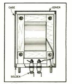
Fig. 7. Typical construction of a sealed transformer. (Courtesy Thordarson Elec. Mfg. Co.)
