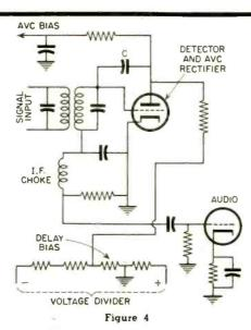
a.v.c. This circuit which is illustrated in *Fig.* 4 prevents a.v.c. from acting until a definite input is achieved and permitting it to act at all greater inputs. The characteristic of such a circuit is shown by curve C of *Fig.* 3.
