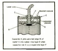
Fig. 2. Another method of using a laminated gasket on a tubular capacitor. (Courtesy Stupakoff Corp.)
