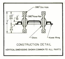
Fig. 4. Multiple conductor glass-to-metal terminal. (Courtesy Stupakoff Corp.)
