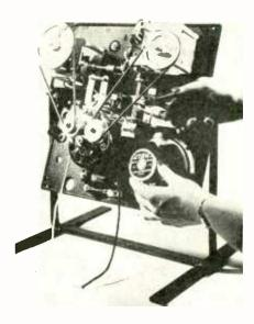
capable of making recordings on a moving steel wire and reproducing them immediately. It accomplishes this by producing small magnets along the moving wire according to the frequency and intensity of the audio signal, and converting the "peaks" and "valleys" of the moving magnetic field thus produced into sound by suitable electrical and mechanical means.
