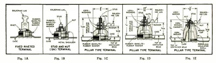
Typical terminal constructions used in sealing capacitors and transformers. (Courtesy Aerovox Corp.)
