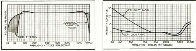
Fig. 11. (Above left) Amplifier having desirable sharp cutoffs. Fig. 12. (Above right) Compensation required over volume limits in the home. Listener on axis of speaker
