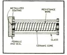
Fig. 8. New type of sealed resistor construction.
