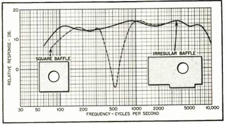
Fig. 10. Effect of baffle on sound pressure curve
