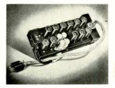
and a half-power bandwidth of 9.0 mc. An external gain control is easily provided. Unless otherwise specified, a standard 500 ohm input impedance is supplied. The output stages are cathode followers designed to operate into impedances of 75 to 100 ohms with voltages ranging from 0.5 to 2.0 volts, negative or positive.
