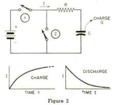
refer to Fig. 2, in which a capacitor is charged through a resistor with a suddenly applied d-c voltage and then discharged through the same resistance. If switch 1 is closed and switch 2 is open, we have:
