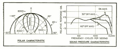
Fig. 8. Polar distribution of sound for typical speaker
