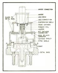
Details of General Electric type 2C40 lighthouse tube, showing method of sealing terminals
