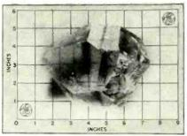
(General Electric photo) Fig. 1. Typical peak prismatic type raw quartz crystal
