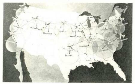
Airborne television and FM broadcasting system. This system, developed jointly by Westinghouse Electric Company and The Glenn L. Martin Compan, proposes to beam (solid lines) programs originating in ground studios to planes for broadcast. Similarly beamed plane-to-plane connections (dotted lines) would form a nationwide network
