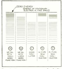
Fig. 4. Characteristic energy level diagrams for various kinds of materials
