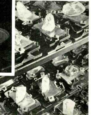
tion to the upper plate. This machine comprises a type of optical lap and is illustrated in *Fig.* 2. One advantage of this machine is the large number of blanks that may be lapped at a time.
