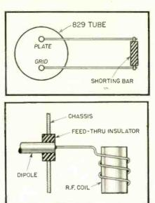
Fig. 4. Typical design applications of aniline laminates: shorting bar and feed-thru insulator
