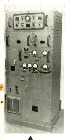
Raytheon SG Main frame. This unit comprises the main component instruments of the radar apparatus
