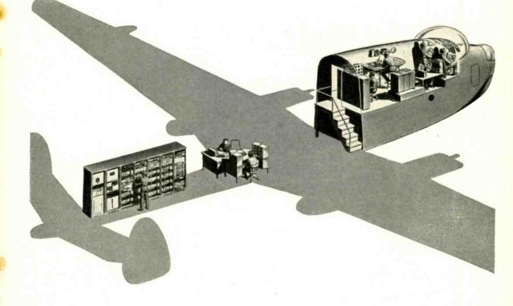
This is a "flight trainer"— an electronically operated replica of the PBM-3 flying boat. It was conceived by the Bureau of Aeronautics and developed by Bell Telephone Laboratories to train Navy bomber crews on the ground.
