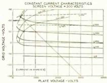
4-125A constant-current characteristics. The operating line (short dashes) Illustrates α 3000-volt. 500 watt input. 75 percent efficiency operating condition
