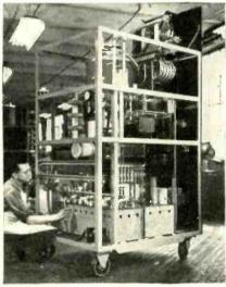
lligh frequency induction furnace used in all radio tube plants where exhaust machines operate. Made by Sylvania Electric at Williamsport, Pa.
