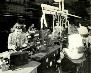
(North American Philips photo) Fig. 4. X-Ray orientation machine
