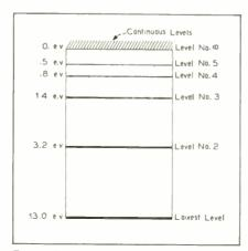
Fig. 3. Energy diagram of hydrogen atom
