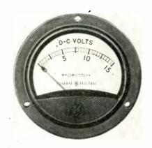
ments, for direct-current voltmeters and ammeters and for a-c radio-frequency ammeters, can be furnished in all standard ratings mentioned in, and conform to the performance requirements of, American War Standard ASA Specification C-39.2-1944. They especially meet the urgent demand of the Armed Services for moisture—and fungus-proof indicating instruments so vital for long-time service under tropical climatic conditions.
