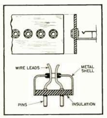
Fig. l. Typical design uses of melamine laminates. Telephone jack panel board (above), and plug insulation
