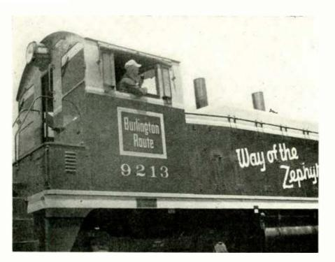
Radio equipment on 1000 H. P. Diesel switch engine. Engineer holds differential microphone
