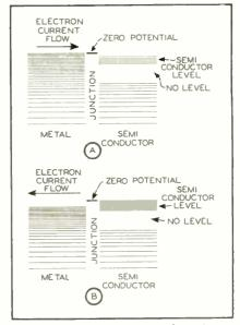
Fig. 5. Energy level diagrams of two types of rectifying junctions
