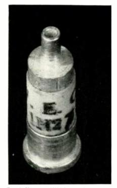
Fig. 2. The type 1N21-B crystal, a typical example of modern crystal rectifier construction
