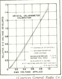
Fig. 6. Curves of average characteristics of 20 crystals
