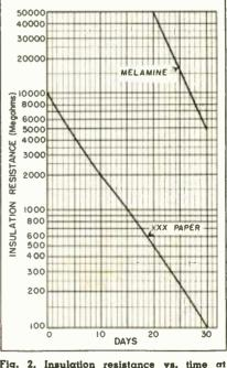
Fig. 2. Insulation resistance vs. time at  $40^\circ$  C. and 90 % R.H.
