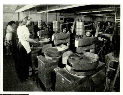
(Above) Fig. 2. Bank of optical laps' (Bliley Electric Co. photo)
