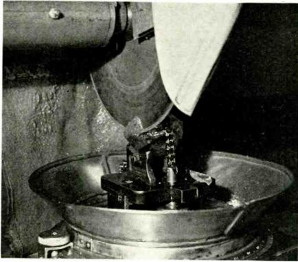
(Above). Close-up view of saw blade cutting end off raw crystal (North American Philips photo)
