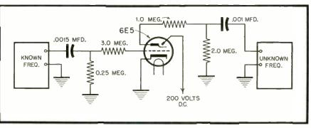
Fig. 2. Schematic of simple indicator for matching frequencies
