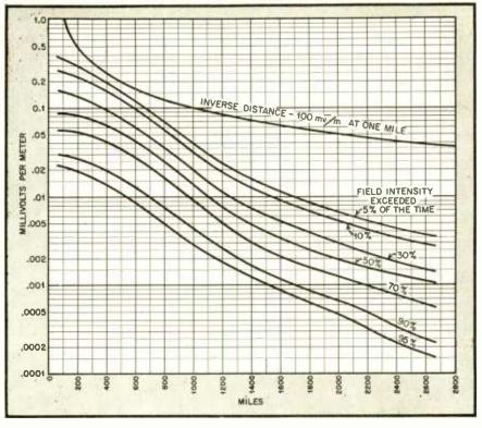
Fig. 5 Propagation curves of sky wave
