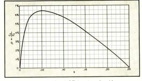
Fig. 4 Plot of the ratio Zt/R for various values of k
