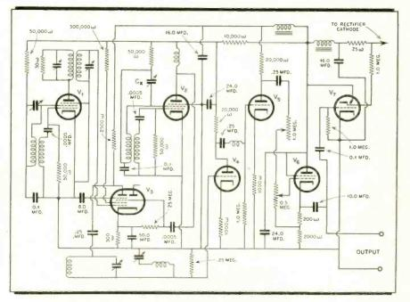
Fig. 5 Audio frequency oscillator
