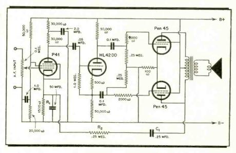
Fig. 4 Negative feedback amplifier
