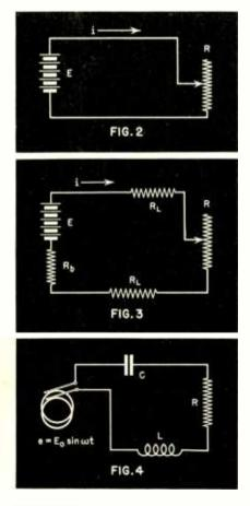
no physically realizable leads from the battery to the resistor with zero resistance. Fig. 3 is the actual circuit. It is well to bear in mind, then, that when the apparent circuit does not behave as it should, a search for the real circuit should be instituted.
