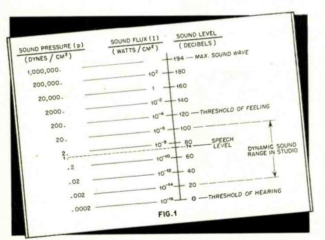
Inter-related sound-pressure, sound-flux and sound-level scale.
