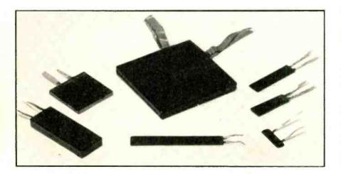
Fig. 4. Typical "Bimorph" crystal elements completely fabricated.
