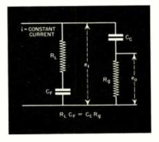
Fig. 4. Equivalent of low-frequency circuit.
