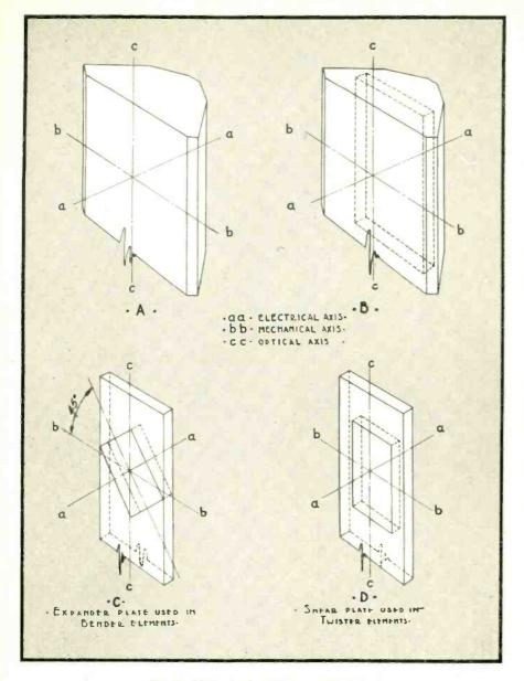
Fig. 2. Method of cutting crystal plates.
