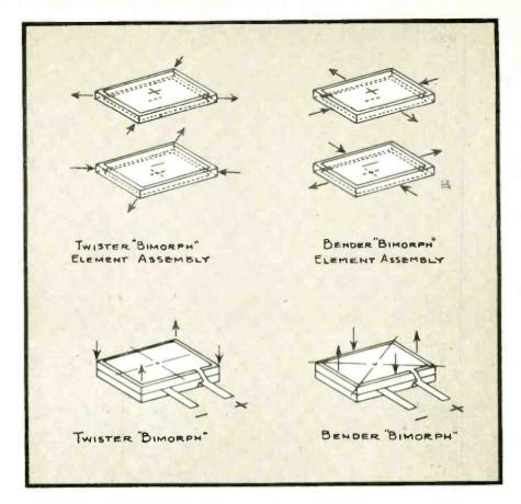
Fig. 3. Construction of "bender" and "twister" "Bimorph" elements. At top are single electroded plates in their relative preassembled positions. Arrows indicate the directions of maximum instantaneous strains for the indicated applied voltage polarity. In the lower sketches the arrows indicate the location and direction of maximum motion of the element relative to the indicated axes.
