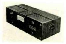
Frequency is indicated directly on front panel of meter or on separate recorder. The meter has an input impedance of 100,000 ohms or over. It will measure trequency regardless of input signal voltage variations between  $\frac{1}{2}$  and 200 volts. Stability is maintained with line voltage variations between 105 and 125 volts.
