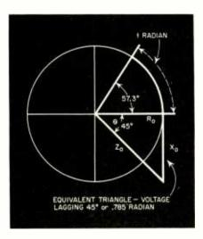
Fig 3. Sketch illustrating phase shift.
