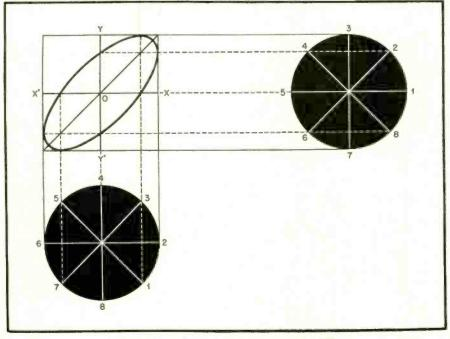
Fig. 4. Phase difference  $= \pi/4$ . Result: Ellipse.
