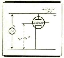
Fig. 7. Grid and plate voltage relation
