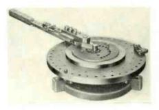
Accuracy guaranteed to tolerance of .001" in all duplicate work. Right or left hand mounting or operating. Automatic and reversible forming nose. Length of operating leverage is 35". Increased lev-erage up to 80" may be added. Capacity,  $\frac{1}{2}$ " round cold rolled steel bar, formed cold to 1" radii or larger. Catalog sheet available on request to
