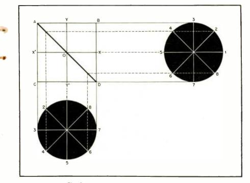
Fig. 2. Phase difference  $= \pi$ . Result: Line AOD.
