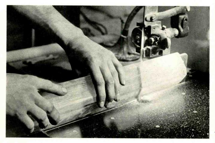
Fig. 1. Slab of Rochelle salt being cut from large homogenous bar.
