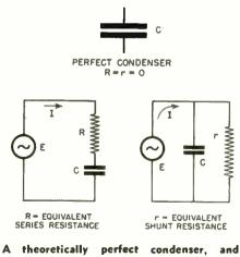
A theoretically perfect condenser, and equivalent circuits representing series and shunt resistance. factor capacitor; i.e., the formula required to convert from one to the other.
