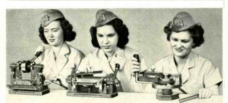
SHEARS l)I-Acro Shear squares and sizes material, cuts strips, makes slits or notches, trims duplicated stamplings. Shearing widths  $-6^{\sigma}$ , 9", 12".
