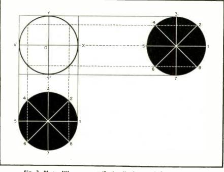
Fig. 3. Phase difference  $=\pi/2$ , Amplitudes equal. Result: Circle.
