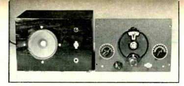
This simple 20-160 meter superheterodyne may be constructed for about \$20, and will give excellent results. The power supply and speaker are housed in a plywood box of the same approximate size as the receiver proper.
