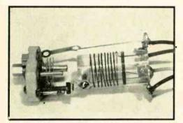
Figure 1. One of the coils used at  $L_1$  and  $L_2$  shown removed from its shield can. These coils are wound on 1/2-inch polystyrene coil forms. The closed end of the form was drilled and tapped on the side to take a 6-32 brass screw. A small angle bracket and a 4-40 by 11/2-inch bolt holds the coil form to the trimmer condenser.
