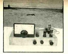
10 to 21/2 meter superheterodyne of W6SLO. Using the new "button" u.h.f. tubes of the 9000 series, it provides excellent reception on both f.m. and a.m.
