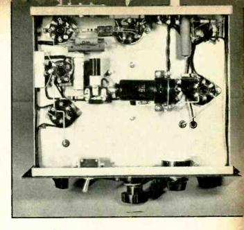
Under-chassis view. The 6K8 is mounted so as to permit the shortest possible grid lead. The "peaking coil," wound on a piece of wood dowel, is mounted at least a half inch away from the chassis and any other components.
