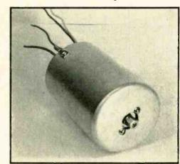
Figure 2. One of the 9-meter coils shown installed in its shield can. The holes in the top of the can were hand made to fit the condenser mounting holes. Figure 3. The receiver installed in its cabinet. The knob on the left actuates the volume control and the on-off switch. On the right is the squelch control.
