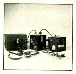
Figure I. The complete field unit for dry-battery power. The universal SW-3 is on the left, the battery box (which houses the batteries for both transmitter and receiver) is in the center, and the c.w. transmitter is on the right. All are described in the text.
