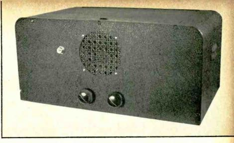
both frequencies. These three features can be listed as "musts" for such a receiver: crystal control of the h.f. oscillator, automatic volume control, and a good signal-to-noise ratio. The front end of any superhet receiver is always improved by the use of a preselector stage, so one was incorporated into the design of this superhet.
