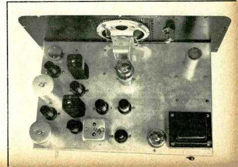
Figure 4. Top view of the finished receiver. The antenna post for 2414 kc. is on the front of the first i.f. can. fourth harmonic of a 7041 kc. amateur band crystal beating with a 30,580 kc. signal gives an i.f. of 2414 kc. (A higher-than-signal frequency crystal is available at about three times the cost of the amateur band crystal.)
