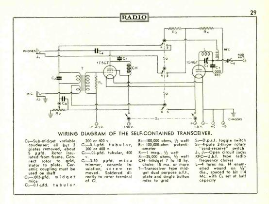
moved from the cabinet). Insert the microphone and earphone plugs, making sure to get them in their correct respective jacks. It is possible to hear very weakly with the phones in the mike jack, but needless to say it is impossible to transmit with the microphone in the earphone jack. No damage will result if the two plugs are accidentally transposed.
