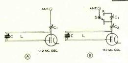
Figure 1. Simplest method of permitting optimum antenna coupling both on send and receive, applicable only when capacity coupling is employed, is shown at "B".
