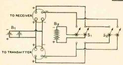
Connections inside the portable battery box. S1-D.p.d.t. toggle switch, plate voltage to transmitter or receiver S2-D.p.s.t toggle switch, standby switch for transmitter or receiver B1-1/2-volt A battery, two dry cells or 4FH's in parallel B2-90-volt B battery, two 45-volt Z30N in series
