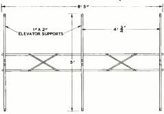
Figure 3. Detail drawing of the phasing section and the Q bars.
