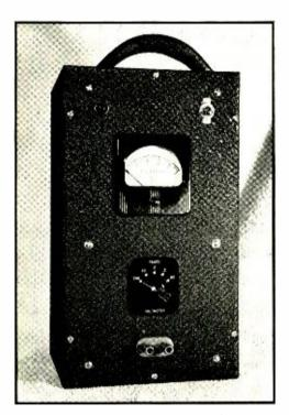
Figure 1. Front view of the v.t. voltmeter. The case is one intended for transceivers. The a.c. switch and pilot are at the top of the panel; the input terminals at the bottom. To most amateurs a vacuum-tube voltmeter is an instrument—made up of an expensive microammeter and a collection of odds and ends—for which the calibration curve has been lost. In other words the usual vacuum-tube voltmeter is nice to have, expensive to get, and not used much anyway.
