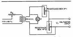
Figure 5. Circuit for calibrating the lower ranges.  $R_s$  is adjusted for a reading of 2 volts on V.  $V_1$  will then be equal to the resistance across the terminals of box 2 times .001. The sum of the resistances of the two boxes should be 2000 ohms at all times.
