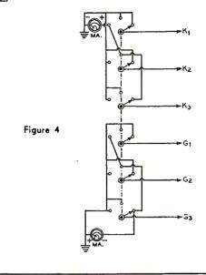
be made by Ohm's law, and the switch must be of the non-shorting type.
