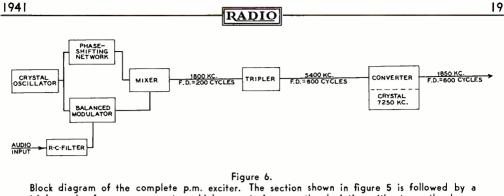
tripler and a frequency converter, which serve to increase the deviation without greatly changing the output frequency.
