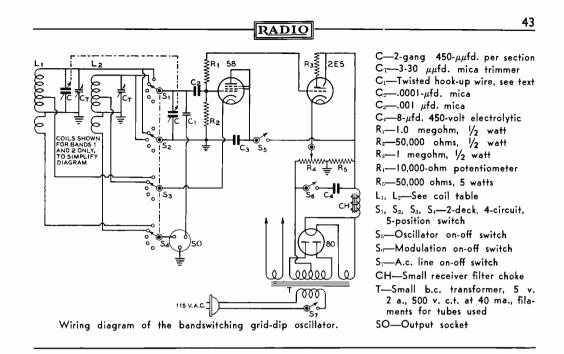
was measured by a meter reading rectified grid current; since then the introduction of the electric eye tube has simplified the operation of the instrument by eliminating the meter movement inertia which sometimes obscured small dips.
