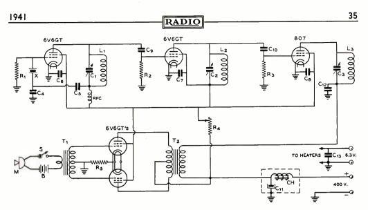
Wiring diagram of the transmitter. It may be used either as a fixed-station transmitter on 28 or 56 Mc., or as a mobile transmitter on 56 Mc.
