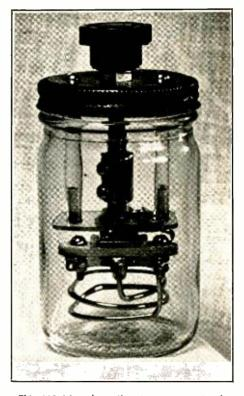
This 112 Mc. absorption type wavemeter is mounted inside a Mason jar to preserve the accuracy of calibration. There is no danger of getting "bit" when the meter is brought near a high power tank circuit.
