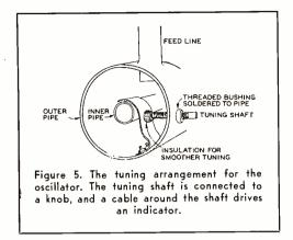
to the cold end of the pipe. This filament lead is insulated from the inner conductor by a thin sheet of mica. Equal results can be obtained with the filament lead down through the inside of the inner conductor by drilling a hole in the  $\frac{1}{2}$ -inch pipe near the cathode connection. If this type of connection is used the filament wire will have to be by-passed to ground at the cold end of the pipe.
