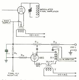
Schematic of the Negative-peak Overmodulation Indicator
