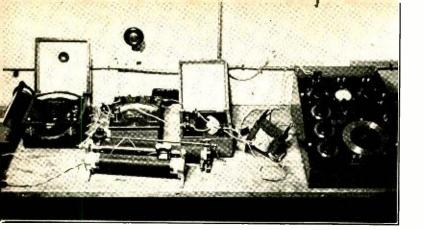
Figure 1. Laboratory set up to measure effect of flux density upon coil and core loss.
