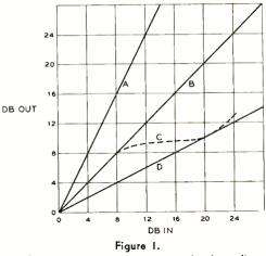
Illustrating various input-output level amplifier characteristics. Curve B is that of a normal amplifier. Curve C is that of the compression amplifier of figure 2.
