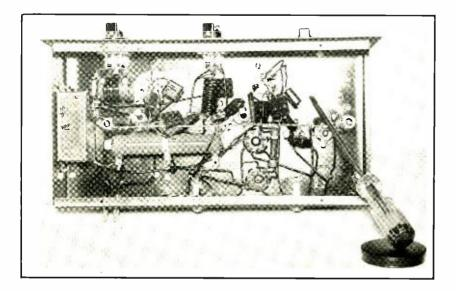
Figure 3. Underchassis view of the transmitter. Notice the common ground bus running down the center of the chassis. The 14- and 28-Mc. coils can be seen mounted upon their respective tuning condensers.
