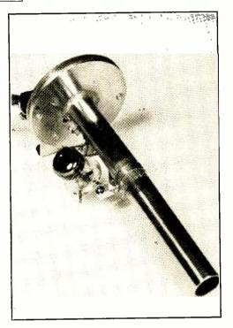
Figure 7. The oscillator with the outer conductor of the concentric line removed; these insides can be removed easily by disconnecting the plate connection and then sliding the works out. Note particularly the grid condenser and the filament-cathode connection.
