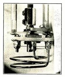
A closeup view of the wavemeter, illustrating detail of construction. Note the lucite posts.
