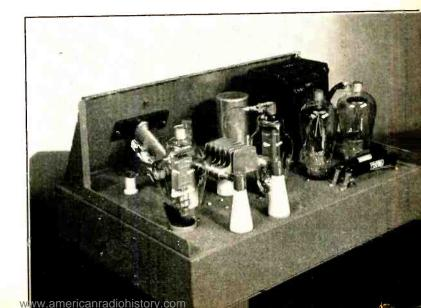
Rear three-quarter view of the chassis with the cover removed. This photograph shows the construction of the homemade plate tank condenser and the method of mounting the pad tuning condenser.
