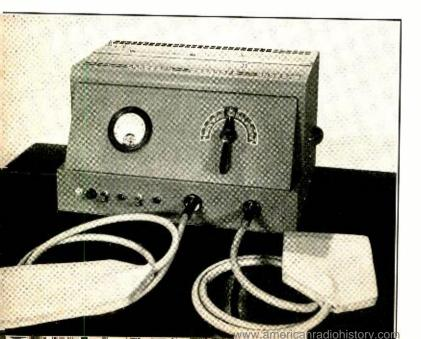
The case for the diathermy unit has handles mounted on the side to make for easy portability. Along the front drop of the chasis are the following: overload relay reset, fuse container, filament switch, green (filament) light, plate power switch, red (plate) light, and the two output jacks for the pads. Top view of the chassis of the unit with the cover to the case removed. Since this photograph is taken dead-on, it gives an excellent idea of the top-chassis layout of components.
