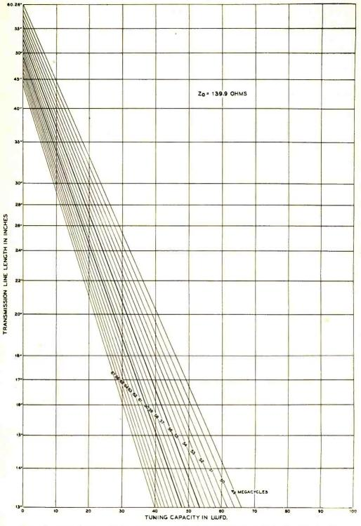
Figure 2. Chart showing capacity necessary to resonate shortened lines of 139.9 ohm surge impedance.
