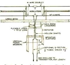
Figure 5. Transmission line connection to 4-wire doublet.
