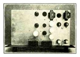
Figure 4. Looking down upon the chassis. The large space to the left is for possible future use as a mounting for a variable-frequency oscillator unit for transmitter control.
