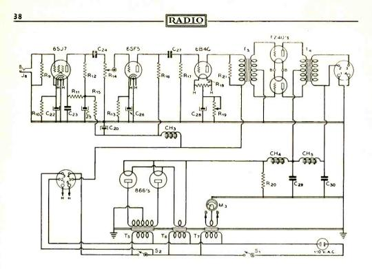
Schematic of the speech, modulator, and the high voltage power supply.
