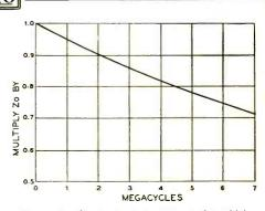
Figure 4. Chart showing constants by which mixer line surge impedance can be multiplied in order to obtain oscillator line surge impedance for tracking with lines of the same length.
