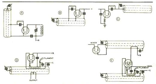
Figure 5. (A) concentric line tuned grid, coil tuned plate oscillator. (B) cathode-above-ground type oscillator circuit with concentric line. (C) single control oscillator circuit without tap on line, although stability can be increased by tapping the grid down. (D) RCA's oscillator circuit used in a broad band transmitter having good stability, requiring only one tuned circuit. (E) similar to (D) but showing pentode tube and balanced loop coupling to mixer stage. 17
