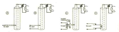
Figure 6. (A) coupling a concentric line feeder to a concentric line resonant circuit. (B) unbalanced method of coupling two wire line into a concentric line circuit. (C) balanced-to-unbalanced method of coupling a two wire line to a concentric line resonant circuit. (D) balanced loop method of obtaining good coupling from two wire line to a concentric line circuit.
