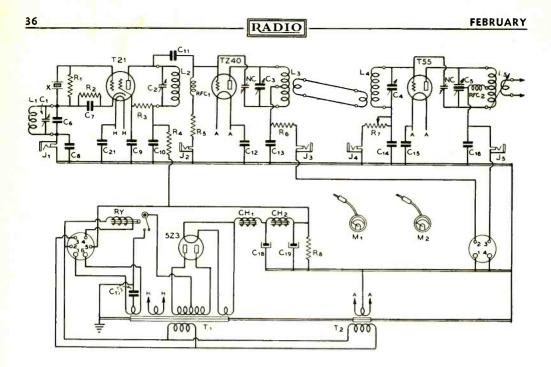
Wiring diagram of the r.f. section and the low voltage power supply.
