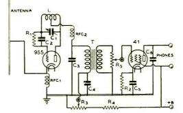
Figure 3. The 112-Mc. receiver circuit used by Kay Sheffer, W9CQV, showing the unusual method of cathode antenna coupling. Note that the r.f. section is mounted upon a piece of lucite.
