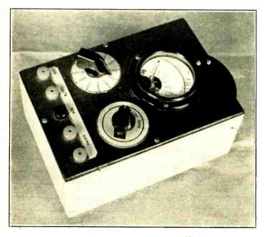
The completed multi-tester mounted in its cabinet. The panel is made of tempered presdwood and the box itself is of pine, lacquered to give a smooth durable finish. This type of mounting makes for easy portability.
