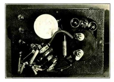
If the panel is unbolted and removed from the box, this is the view that greets the eye. All components of the tester itself have been mounted directly upon the presdwood panel.
