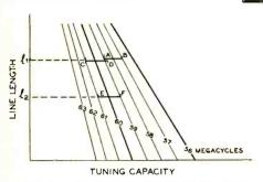
Figure 3. Exaggerated chart similar to figure 1, to illustrate method of tracking oscillator by shortening line, as described in text.
