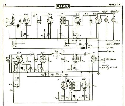
Wiring diagram of the combination modulation monitor and pre-amplifier.
