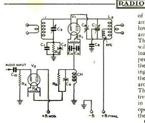
Figure 1. Wiring diagram of a single-ended r.f. amplifier being modulated by a triode parallel cathode modulator.  $R_3$ , by-passed by  $C_9$ , plus the drop across the choke CH furnishes the bias for the modulator tube  $V_2$ .
