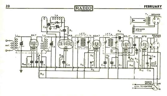
General wiring diagram of the five-tube super.
