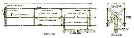
Figure 3. Experimental design of 4-wire doublet.
