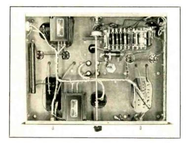
Under-chassis view of the speech amplifier, modulator, and main power supply deck, The speech amplifier components are arranged along the extreme rear of the chassis. Note the use of a large mounting bracket for the volume control and the low-level input stages of the speech amplifier.
