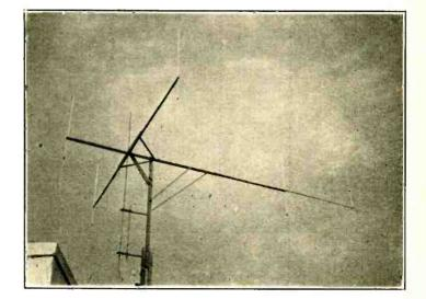
Closeup view of the stub-fed 7-element Yagi array.
