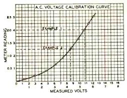
Figure 7. A.c. voltage sample calibration chart. After the chart has been made up for the individual meter it is used as follows: Example 1-meter range, 2500; meter reading, 2000; curve gives actual voltage as 5400. Example 2-meter range, 500; meter reading, 250; actual voltage from curve, 860.
