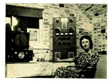
Beulah B. Tolonen operating her station K7GLL at Kennecott, Alaska. The final stage uses a 100TH with 250 watts input on both phone and c.w.
