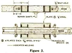
Top and side views of the main mounting plate showing how it is bolted to the boom.
