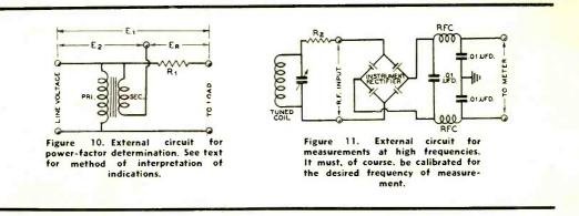
cuit, the writer has developed a method for the determination of power factor which involves only the measurement of voltages. Figure 10 illustrates the circuit diagram.
