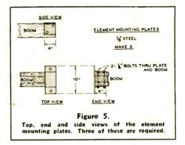
dimension and just far enough apart to allow them to slip snugly over the boom. Each of the 4 x 4 inch pieces had two holes drilled in it to allow it to be bolted to the boom and the large 4 x 12 inch plate had holes drilled near each end to allow bolting the element-supporting cross members to it. A detailed drawing of one of the element mounting plates is shown in figure 5. One of them may also be seen in figure 4 straddling the boom to the right of the main mounting bracket.
