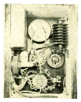
Interior view of the multi-meter. The rebuilt rectifier can be seen on the right-hand wall of the box.
