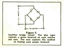
versal meter when each cell was connected in so as to show its higher resistance. The four cells were then connected in the bridge rectifier circuit as shown in figure 6.
