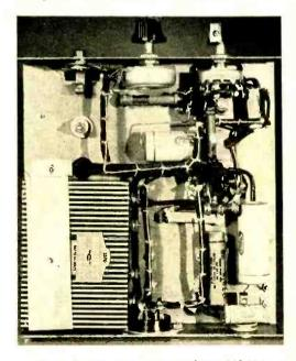
Figure 3. Under-chassis view of the 112-Mc. transceiver. Exact placement of these parts and length of leads between them is not important. All grounds are made to the nearest convenient point on the chassis.
