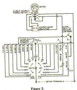
Complete wiring diagram of the multi-meter.
