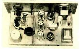
Top view of the improved RC superhet. The can in the lower left corner shields the tuned r.f., choke which is incorporated to increase the i.f. selectivity.
