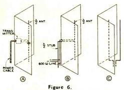
Methods of feeding the driven radiator. The arrangement at C is a single-section flat-top beam with square-corner reflector.
