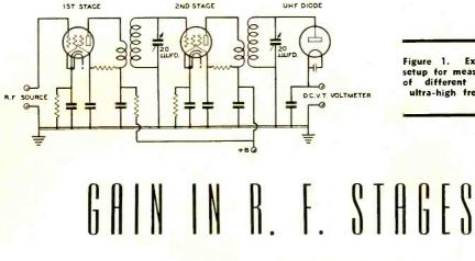
Figure 1. Experimental setup for measuring gain different tubes at ultra-high frequencies.
