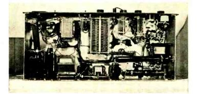
Bottom view of the transmitter. All tank condensers are mounted below chassis; the final tank condenser is the large single-section affair mounted in the center.
