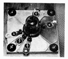
The completed socket with the tube and the capacity increasing plates in place and mounted upon the stage shield.
