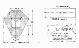
Cloth pattern and constructional diagram of the assembly of the kite.
