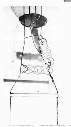
Figure 4. Bottom end of the quarter-wave line of which the upper end is shown in figure 3. The 600-ohm transmission line leaving the end of the matching section can be of any reasonable length.
