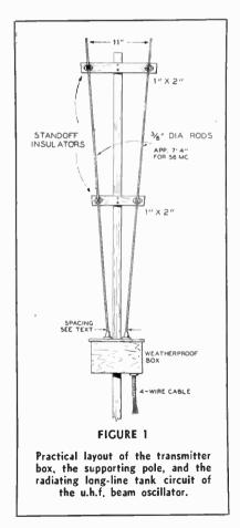
A simplified type of oscillator or final amplifier for use on ten meters and below has been developed by Bob Smith, W3HJO. With it, he has put an R7 signal into Baltimore from Washington with 4 watts input and the antenna indoors, while with 60 watts he has raised all districts but W6 and W7, on five meters.
