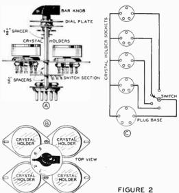
Horizontal type assembly whereby the multiple holder and the selector switch are both plugged into the original crystal socket. The arrangement is shown in (A) and (B) and the method of connection in (C).
