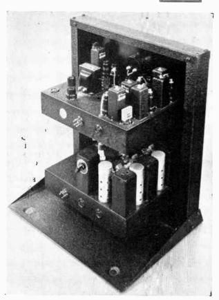
Rear three-quarter view of the completed receiver exclusive of power supply. The interconnecting plugs also have been removed to clarify the photograph
