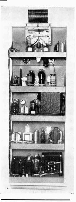
Back view of the complete transmitter with 80meter coils in place. In top to bottom order the units are: final amplifier, exciter, modulator, lowvoltage power supply, and high-voltage power supply.
