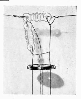
Figure 3. Method of connection of the upper end of the quarter-wave matching section to the center of the antenna. The coding of the wires indicates their polarity. Strain insulators are 3<sup>1</sup>/<sub>2</sub>-inch Pyrex and the circular insulator is a phenolic "glass coaster."
