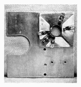
Showing the method of assembling the socket. The cathode and suppressor clips are bolted to the copper sheet.
