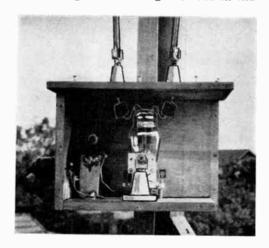
FIGURE 3 Cutaway view of the transmitter box showing the oscillator tube and its grid tank circuit.
