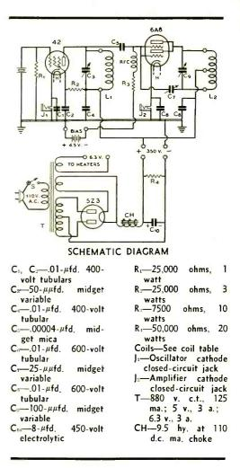
With the lower voltage, 300 volts on both plates, the power output will be reduced somewhat more than proportionately; 12 to 15 watts output can be expected.
