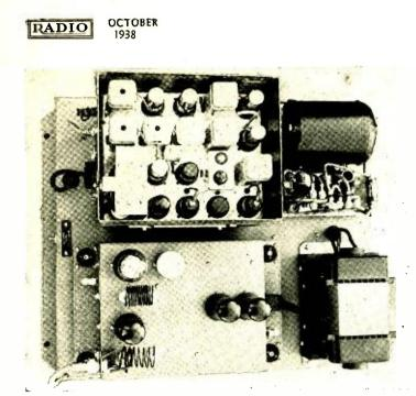
A top-of-chassis view of one of the complete units with the various covers removed. The RCA receiver with its associated power supply can be seen along the top and the four-tube transmitter, mounted upon shock insulators, with its dynamotor can be seen below.
