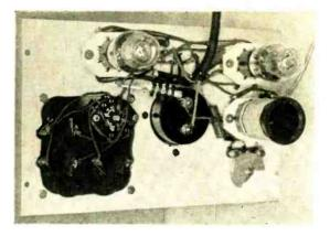
Under-chassis view of the unit. The homemade multiple crystal holder, made from a micarta plate and holder clips, can be seen in the lower left corner.
