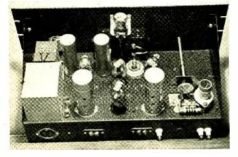
Figure 2. Rear view showing the shielded input circuit on the right, the various other components in the center and the special power transformer and choke alongside the left edge of the chassis.
