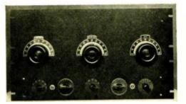
Front view of the bandswitching exciter mounted on a standard rack panel. The controls along the bottom of the chassis are: crystal selector switch, 6A6 doubler plate condenser, exciter bandswitch, final grid excitation control and final plate bandswitch.
