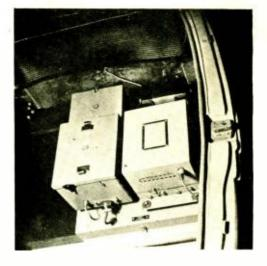
A vertically-mounted installation of one of the units behind the front seat of the Fire Chief's car. The appea ance of the units with their covers in place can be seen in this view.
