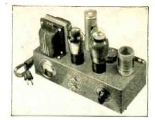
mobile or emergency transmitter. Metal tubes are supplied with the d.c. portable because of their greater ability to withstand hard usage as compared to the glass ones used with the a.c.-operated unit.
