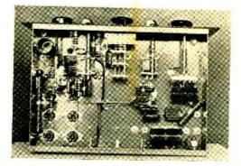
Bottom view of the chassis with all the components mounted but before the major portion of the wiring process has been begun.
