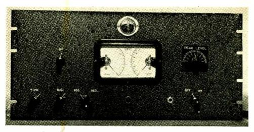
Figure 🧯 Panel view of the rack-mounting type modulation indicator.
