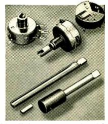
Mallory-Yaxley Midget Volume Controls have flexibility... adaptability... universality... and attachable switches where necessary. But overshadowing all these advantages is the Mallory-Yaxley Plug-In Shaft!
