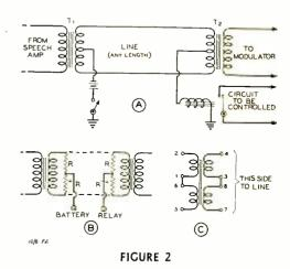
(A) Two-wire line with voice and control over same wires (phantom control circuit).  $T_3$ —Plate-to-500 ohms,  $T_2$ —500 ohms-togrid. (B) Same as A except that resistors are used to determine mid-point on transformers without a center-tap. R—500 ohms (see text). (C) Method of making connections to numbered posts of manufactured simplex transformers to balance out control current in windings.
