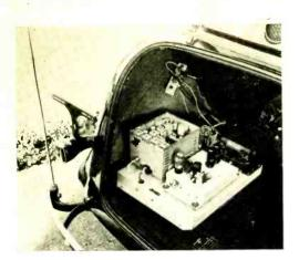
An installation of one of the self-contained mobile transmitter-receiver units as made in the rear deck of one of the new patrol cars of the Beverly Hills, Calif., Police Department. The covers have been removed from the various sections so that they may be seen more clearly. The fishpole antenna with its insulating block can be seen mounted upon the bumper.
