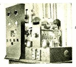
W6CXW showing his new final amplifier with turret tank. The tubes are the same 150T's and the entire exciter and driving unit is behind the panel on the left. Henry used this rig when he worked his 150th country.,
