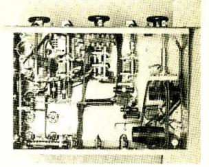
Bottom view of the completely wired exciter. The terminal strip in the upper center of the chassis is for connection to the indicating milliameters
