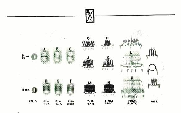
Figure 7. The complete coil complement.
