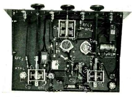
Figure 2. Bottom view of the exciter deck. The various s o c k et s, resistors, c o n d e n s e r s, etc., have been marked to correspond with the schematic diagram.
