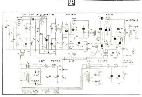
Figure 8. The complete wiring diagram.
