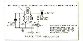
and will immediately start oscillating with no tuning whatsoever. It is an especially handy gadget for aligning a single signal super as the crystal can be removed from the i.f. circuit and put into the test oscillator and the i.f.'s lined up on the nose for the exact crystal frequency used. In almost any other type of crystal oscillator except the Pierce, there is a certain amount of detuning introduced by the oscillator itself.
