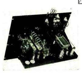
Figure 3. The push-pull T-20 final amplifier.
