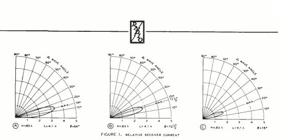
The actual radiated power in each of these lobes is the same; the difference in their apparent size is due to the variation in radiation resistance of the array.
