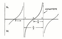
Again, from equation (2), when  $Z_r = \infty$ ,  $Z_s = -jZ_0\cot\beta I = -jZ_0\tan(\pi/2-\beta I)$ . Thus, for  $Z_r = \infty$ , the same relation holds as for  $Z_r = 0$  except that the nodal points, etc., have been shifted by a distance corresponding to  $\pi/2$  electrical degrees or one quarter wavelength.
