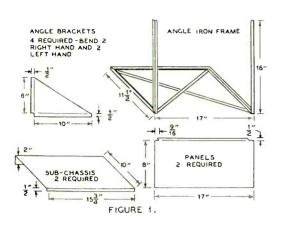
mounted on the rack. The front panels now are laid out for drilling. When the panels have been drilled, they are given a good cleaning and a coat of crystalizing lacquer. Then, reassemble the chassis and panels and mount the sockets, transformers, switches, etcetera. The wiring then may be done in any manner that is convenient.
