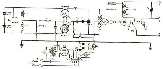
General Wiring Diagram of the Complete Unit
