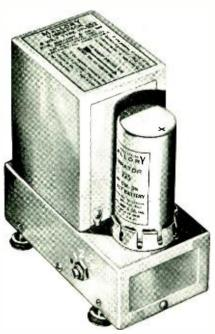
The output of Mallory Vibrapacks is variable in four steps of 25 volts each. The selection of output voltage is obtained through a Yaxley switch connected to various transformer taps. Maximum efficiency is obtained for all load conditions.
