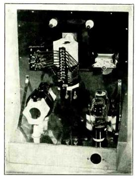
Back view of the r.f. and antenna tuning unit removed from the cabinet
