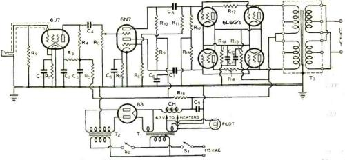
General Wiring Diagram of the Amplifier-Modulator (See Note at End of Article)
