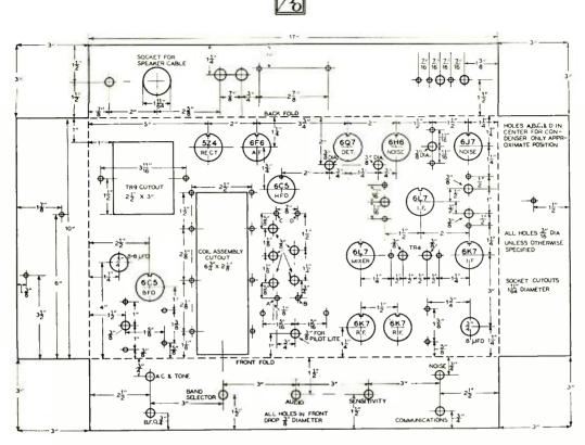
Chassis Layout, Top View (Flaps Bend Down)
