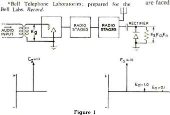
In the output of a radio transmitter there are certain components in addition to the desired signal. These are chiefly a distortion component and a noise component.
