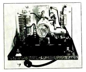
Top Deck of the R.F. Unit, Showing the 6A6 Push-Pull Amplifier
