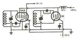
The Revamped 6A8 Converter Circuit
