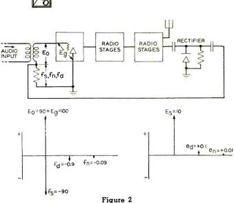
Feedback returns to the input a portion of the output in reverse phase, and in this way cancels part of the output noise and distortion.
