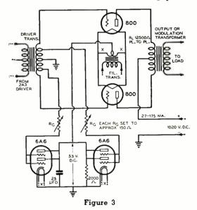
must be provided for the bias tube as well as the power tube grids. This driving power is quite considerable. In some cases, depending on the combination used, it may be as high or even higher than the power tube grid drive needed.
