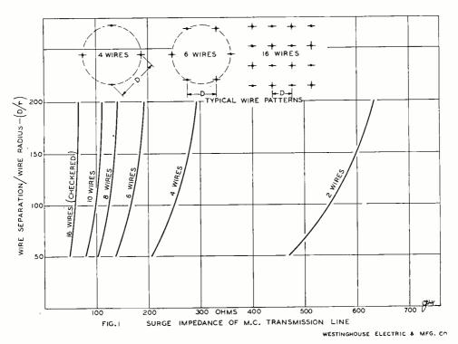
Many of our amateur antenna systems and coupling circuits require radio frequency transmission lines, either as impedance matching transformers or as a connecting medium between the transmitter and antenna system or both.
