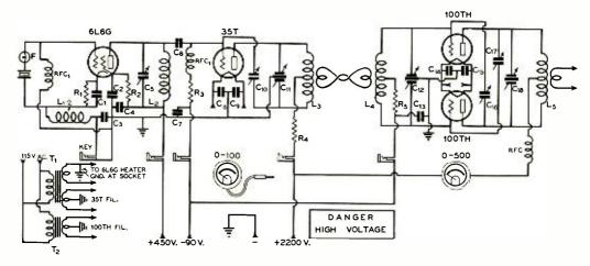
General Wiring Diagram of the 100-TH Transmitter
