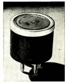
Clarostat Mfg. Co., Inc. These plug-in resistors were originally developed for use in resistance bridges and other test equipment employed in the Clarostat laboratory and plant. Housed in a standard 4-prong tube base, these units are available in values of 1 to 10,000 ohms, with any accuracy up to 1/10th of 1 per cent. Due to the design, they are quite inexpensive.
