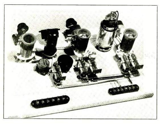
The QRQ-QSY exciter used at W4DHZ. QSYing is done remotely with a single switch by means of relays and padding condensers in the tank circuits.
