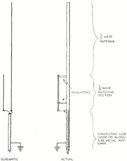
One method used to match a low-impedance line to an end-fed antenna with a matching section.
