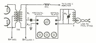
Figure 2: Connections for Trapezoidal Patterns
