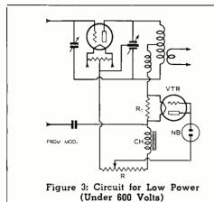
No filament transformer for VTR is needed. Constants same as for figure 1.  $R_1$  is chosen to give VTR (in this case a 30 or 71-A) normal filament current at the plate current drawn by the modulated amplifier.
