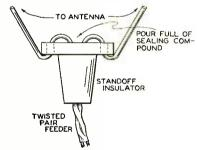
sizes, a suitable size being chosen for the particular feed line to be used. I used a Birnbach type 866-SJ with the hardware removed. After all connections are made, the insulator is poured full of sealing compound. This prevents moisture from getting into the crotch of the transmission line.—W9NBE.
