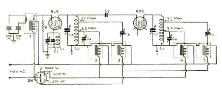
Wiring Diagram of the Exciter, QSY Portion Only
