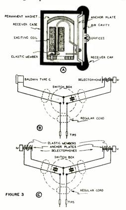
accordance with figure 3-C and located at the Y junction of the telephone cord. The wearer can thus shift from one high selectivity selectophone to the other and utilize the characteristics of either one at will.
