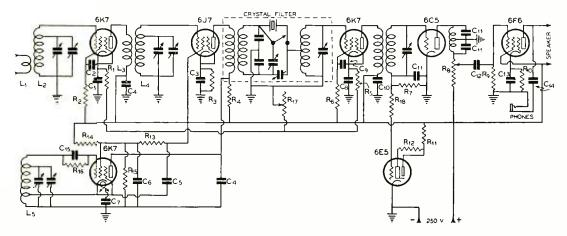
The Bandspread Special 20 Meter Phone Receiver Wiring Diagram
