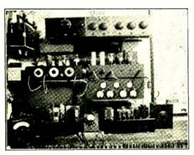
Two transmitters are used at ZUIT. One is used on 20 and 40 meters: the other is for 10. A 66 foot zepp. is used on 20 and 40 meters. A 67 foot single-wire-fed antenna is used on 40, 20, and 10 meters.
