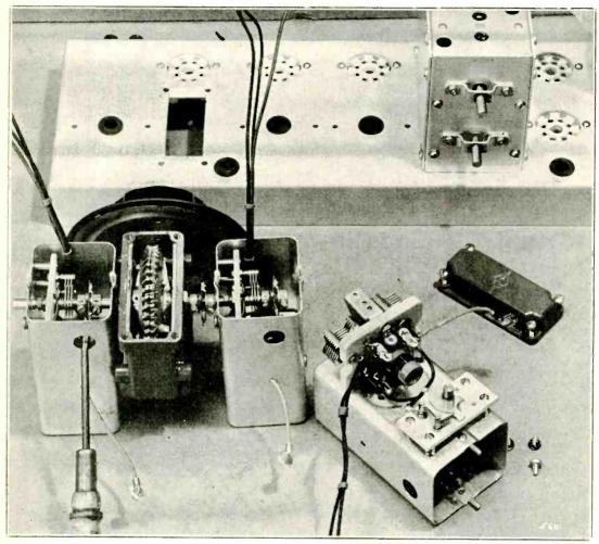
The ganged tuning assembly. Construction can be simplified by using fixed-tune 14.200 kc. tanks for the r.f. and first detector stages and tuning only the oscillator. The resulting loss in efficiency over the narrow phone band is very small, due to the high frequency involved.
