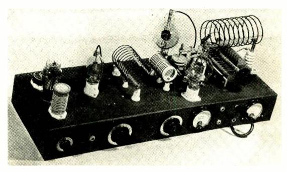
Looking down on the transmitter. The small flashlight bulb connected in series with the crystal is hiding behind the 6L6-G. It is screwed into a small hole in the Masonite and connections soldered to it.
