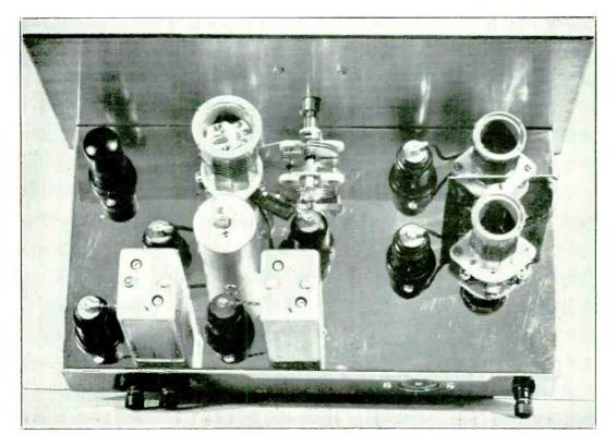
Top View of the "Works". The Blank Space Was Left for a Crystal Filter. To Be Added at a Later Date When the Best Filter Circuit Has Been Determined.
