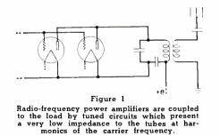
tubes—which is proportional to the product of instantaneous plate voltage and current—will be small, and the efficiency correspondingly high. The efficiency is, in fact, very closely proportional to the amplitude of the plate voltage swing. By permitting the plate voltage to swing down to a value as low as 10 or 15 per cent
