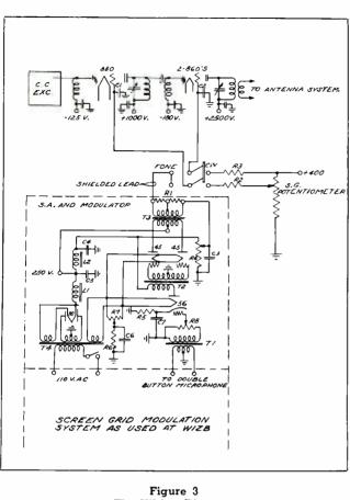
The Wiring Diagram
