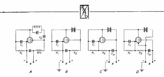
Figure 3 Development of the special crystal oscillator circuit.
