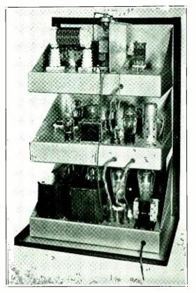
Showing interior construction of the transmitter. It is entirely self-contained.
