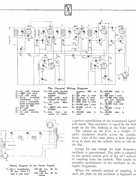
when the cathode method of coupling is used, the plate on the oscillator is bypassed to ground with a small mica condenser of about .01  $\mu$ fd. This type coupling is supposed to reduce oscillator hiss, but when used in a set having separately-tuned r.f. and detector stages (regenerative r.f. stage) there is a slight pulling effect on weak signals when the stages are resonated, unless the coupling capacity is carefully adjusted in each instance, which is somewhat impracticable.
