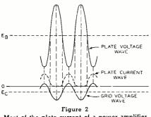
Most of the plate current of a power amplifier flows while the plate potential is in the vicinity of its minimum value, so that the tube loss can be made small by using a plate voltage swing of large amplitude.
