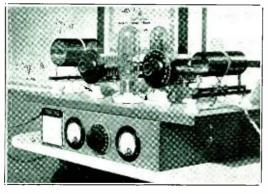
The 500 watt stage. using a pair of carbon plate 203A's in push-pull.
