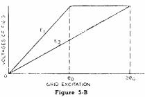
As the grid excitation is modulated about its carrier value  $e_{0}$ , the plate potential of tube V-l does not respond to the positive half-cycles of modulation, since it has reached its maximum value at the carrier output.
