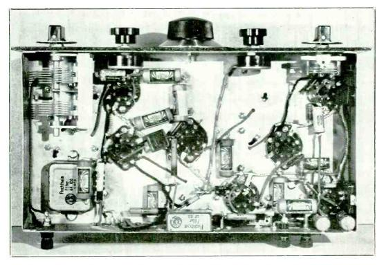
Bottom View of the Receiver. Note the Shielded Wire Used for the "Hot" Filament Lead. The Carbon Resistors Are the New Insulated Type.
