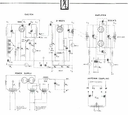
Exciter, Amplifier, Amplifier Power Supply, and Antenna Coupling Unit
