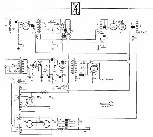
The Controlled Carrier, Suppressor Modulated Phone
