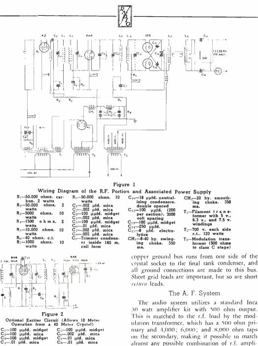
of the modulator. Amphenol Stetite sockets are used throughout, as they are particularly easy to mount directly on a metal chassis. The several "floating" variable condensers are mounted with small angle brackets on midget stand-off insulators.
