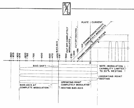
Figure 2 The Class BC Expanding Linear Amplifier, Resting Condition (Axis Shift 33%)
