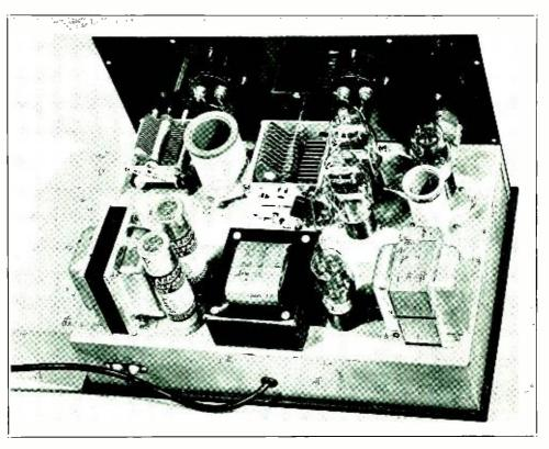
Top View of the 802 R.F. Unit with Cabinet Removed
