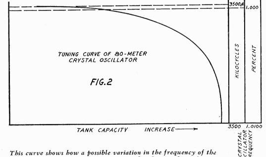
oscillator can be obtained by turning the plate tank condenser.
