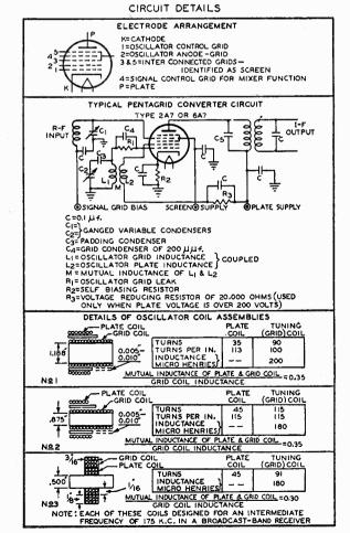
The 1A6 and 2A7-6A7 tubes employ similar circuits and coil design. The above drawing, courtesy of RCA-CUNNINGHAM, will help you in selecting the proper I.F. coils for a super using the 1A6 tube.
