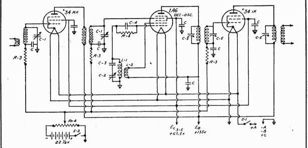
Superheterodyne circuit showing proper use of new 1A6 Pentagrid Converter Tube. The following tubes are required for this receiver: '34 as r.f. amplifier ahead of 1A6; '34's for the intermediate stages; '32 for second detector;
