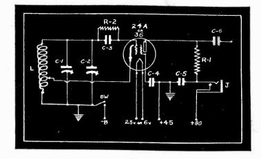
FIG. 2—Conventional Circuit Diagram of an Electron-Coupled Frequency Meter.
