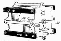
Typical construction of "C" type (Semi-SLW) balanced rotor type gang con-densers. Gang condensers may also be had "straight-in-line" on special order, if desired both "B" (SLC) and "C" (Semi-SLW).
