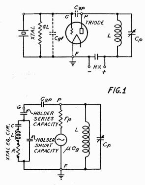
cussion of the voltage effects is that an increase in voltage of the supply lowers the circuit frequency and vice-versa.
