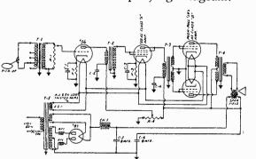
List of parts for Phonograph Amplifier: T-1 Transformer matching pickup imped-
