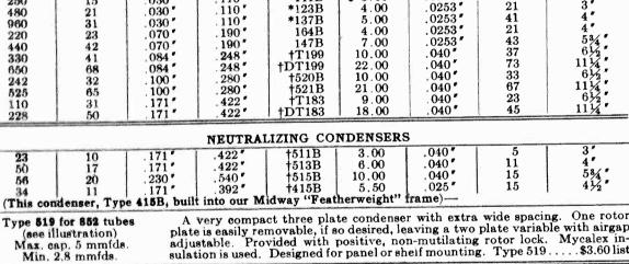
A very compact three plate condenser with extra wide spacing. One fotor plate is easily removable, if so desired, leaving a two plate variable with airgap adjustable. Provided with positive, non-mutilating rotor lock. Mycalex in-sulation is used. Designed for panel or shelf mounting. Type 519.....\$3.60 list
