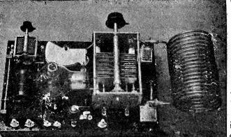
of the grid coil. Since this side is at ground potential, the very bothersome trouble of hand capacity will be eliminated. The plugs on the large tank inductance are the newest types made by General Radio and differ from their previous plugs in that they have a hole in the end that will take up to 5/16-in. tubing. They come filled with solder and all that is necessary is to sweat the tubing to the plug.
