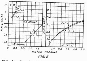
FIG. 5: Sample 1000-cycle calibration for high range, with and without 2-mfd. shunt condenser.
