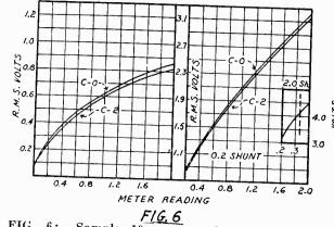
FIG. 6: Sample 1000-cycle calibration for low range, with and without 2-mfd. shunt condenser.
