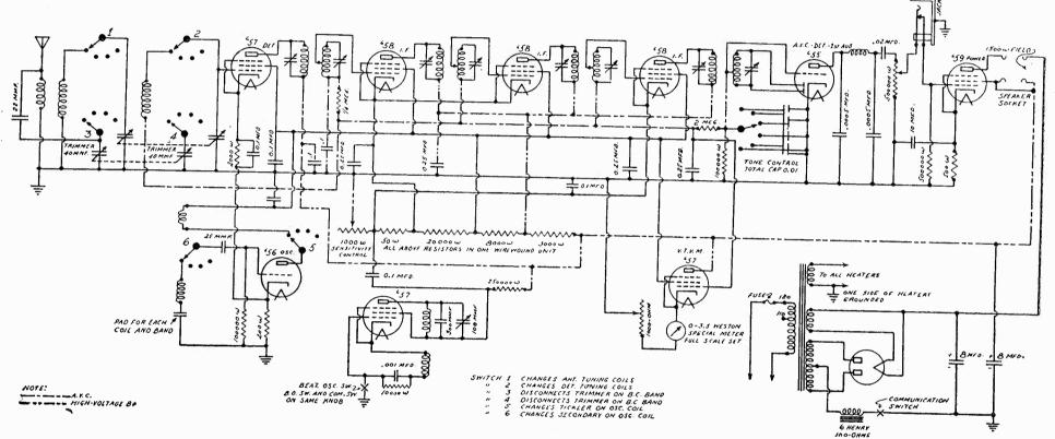
four sets of coils in the conventional tickler feed-back circuit. By inserting a 22Mmf. condenser in the grid circuit of the oscillator, we are able to get a rising characteristic of the oscillator current. In other words, the oscillator puts out approximately four times more energy on 20 meters than it does on the low frequency end of the broadcast band.
