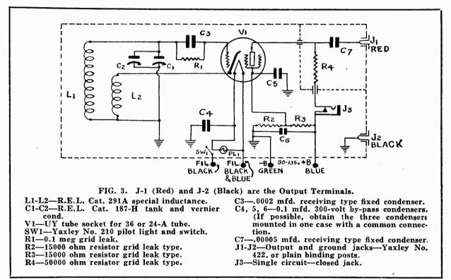
condenser, preferably of the tank and vernier type, is to be desired. A condenser of this construction permits the placing of a lumped capacity across the inductance so that the vernier will give wide spread tuning over the band desired. Choose a condenser having heavy plates as they are less likely to bend, due to slight jars in handling.
