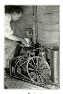
Fig. 3. Application of Filterette 110 to a commercial refrigerator.
