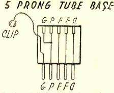
the alarm bell. In practice it was found that the relay could be adjusted to a point sensitive enough to allow a 20,000 ohm resistor connected from cathode to filament of a tube to set off the alarm.
