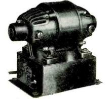
d-c only. It develops 60 watts of 110 volt 60 cycle alternating current and its consumption is only 4 amperes. It is designed specially for the operation of a-c midget sets on 32 volt farm lighting systems. Price, \$49.50 list.
