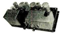
four of the new multi-mu tubes and two pentodes in the power stage. The receiver is said to be non-radiating and contains nine tuned circuits. A local distance switch is provided, not for the purpose of making the set more sensitive for distance reception, but for the opposite purpose of cutting down the sensitivity if the receiver is used within a mile or so of a powerful broadcasting station. A new shadow dial is incorporated in the set which has been designed to completely eliminate paralax.
