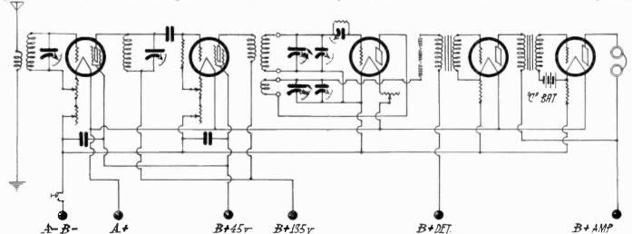
Fig. 1. Circuit Diagram for All-Short-Wave Receiver with Screen-Grid R.F. Amplifier
