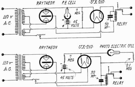
Circuit Diagrams for a Photoelectric Power Amplifier
