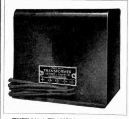
The General Radio Type 565 Power Transformers consist of two models for both half and full-wave rectification utilizing the 281 type of rectifier tube. The Type 565-A Half-Wave Transformer illustrated consists of one 600volt secondary, two secondaries of 7.5 volts and one of 2.5 volts. It is designed for 105 to 125-volt, 50 to 60cycle lines.
