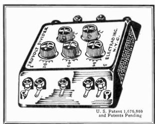
THE Truvolt Divider offers the radio engineer or builder of eliminators for the first time a complete wire wound resistance unit so arranged with five adjustable contacts that all required voltages may be obtained with any set or eliminator combination.
