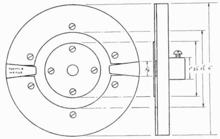
Fig. 3. Commutator Disc
