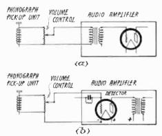
Fig. 1. Usual Methods of Connecting
