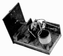
Wavemeter with Neon Tube Indicator
