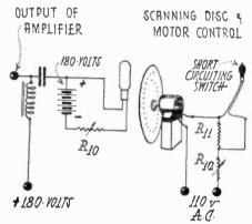
Fig. 1. Circuit Diagram of Television Receiving Equipment
