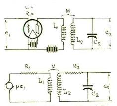
Fig. 1a. Circuit Diagram of Typical R.F. Amplifier Stage. Fig. 1b. Circuit Equivalent of Fig. 1a.
