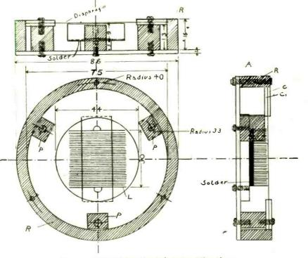
Fig. 1. Structural Details of Capacity Microphone.
