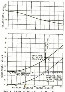
Fig. 6. Effect of Variation in Coupling on Secondary Resistance and Selectivity. tance of the secondary is given by the equation
