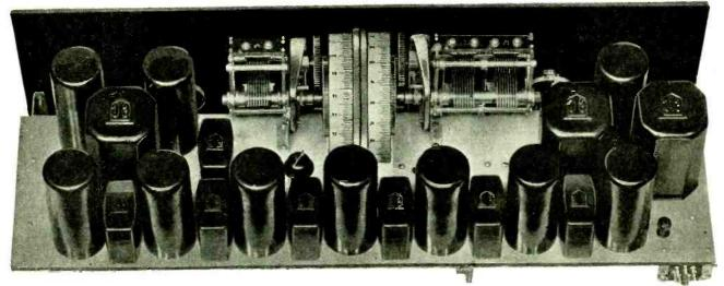
Rear View, Showing Tube Shields.
