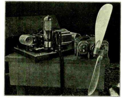
Radio Transmitter and Generator, Ready for Installation on "Dallas Spirit."
