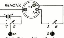
Fig. 1. Diagram of Connections for Continuity Tester.
