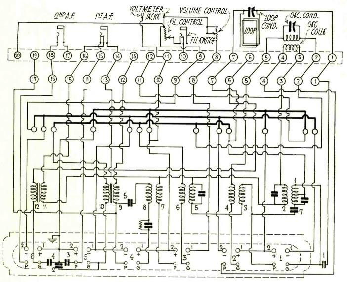
This procedure is best illustrated by actual examples. Fig. 5 is the continuity diagram of a Radiola 25 and Table I is the test sheet to be used with it. As trouble is most likely to develop in the audio circuit the audio coil tests are marked with X so that they may be made first and possibly obviate the necessity of making the others.
