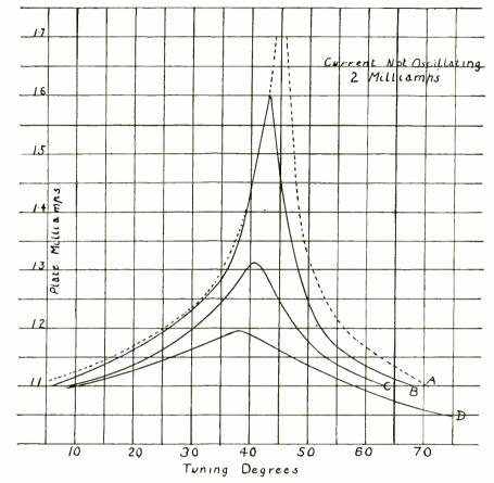
Fig. 2. Resonance Curves of Coupling.
