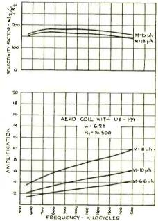
Fig. 11. Performance of Coil With 199 Tube.
