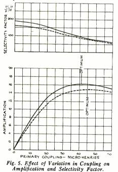
lower Fig. 5. It will be noticed that the amplification rises very rapidly as the coupling is first increased and then reaches a maximum with a coupling of 41.2 microhenries. This value of optimum coupling is given by the equation
