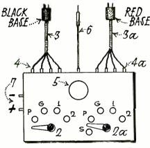
Fig. 1. Pictorial Diagram of Test Box.
