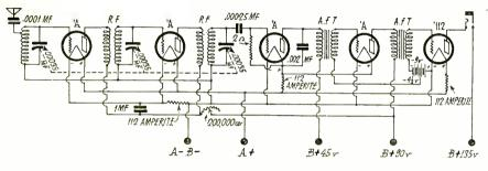
Fig. 1. Circuit Diagram for Five Tube Doughnut Coil Receiver.
