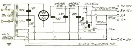
Fig. 2. "ABC" Eliminator Circuit for Magnaformer 9-8.
