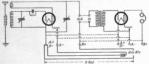
Fig. 1. Circuit Used at Ch-9TC, Showing Position of Leads.
