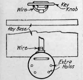
Fig. 3, Simple Connection for Hearing What You Are Sending.
