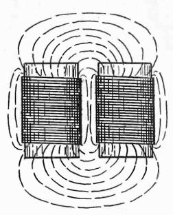
Fig. 2. Electromagnetic Field of Astatic Pair.
