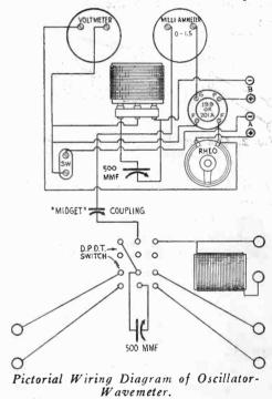
cedure is as follows: With the oscillator in operation and the upper switch to the right, set the unknown condenser, say, at 10 degrees. Throw the external switch so that the oscillator is connected to this condenser and adjust oscillator dial carefully until resonance is indicated by a "dip" (toward zero) of the ammeter pointer. The small coupling condenser should be set so that this dip is very slight—about one division is sufficient.
