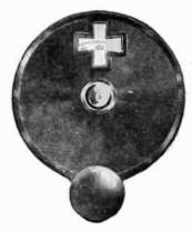
slip or back-lash. It can be used on either clockwise or counter-clockwise shafts. The reading plate has black letters on a satin-finished white metal disk.
