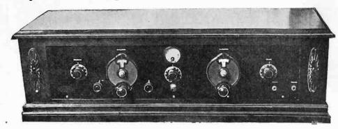
Fig. 1. Front View of Sargent-Rayment Infradyne.
