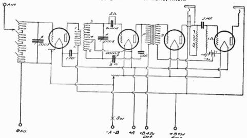
Fig. 3. Circuit of Four Tube Regenerative Receiver.
