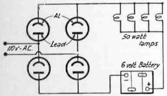
Fig. 1. The Electrolytic Battery Charger Circuit.
