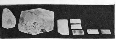
Fig. 1. Various Steps in the Production of a Finished Crystal.
