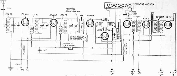
Fig. 4. Schematic Wiring Diagram.
