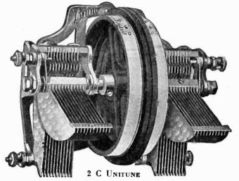
This basic Unit consists of two .0005 mfd. bakelite shaft condensers, controlled by a split drum with graduated scale, mounted in an aluminum frame.
