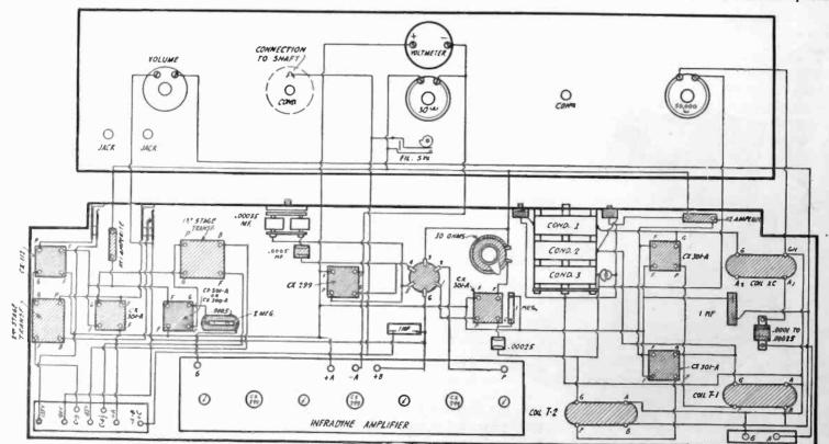
Fig. 5. Pictorial Wiring Diagram.
