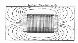
Fig. 5. Shielded Solenoid.
