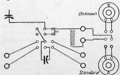
Fig. 1. Connections for Condenser Calibration.
