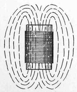
Fig. 1. Electromagnetic Field of Solenoid.
