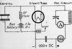
Fig. 6. Crystal Testing Circuit.
