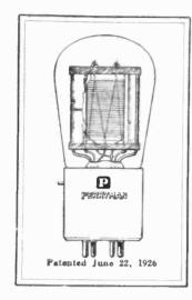
has the patented bridge and double filament advantages of Perryman Tubes. The patented bridge insures Perryman Tubes against jars and jolts and keeps the elements in place. The double filament means double efficiency and longer life.
