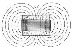
Fig. 4. Field of Short Coil with Large Diameter.
