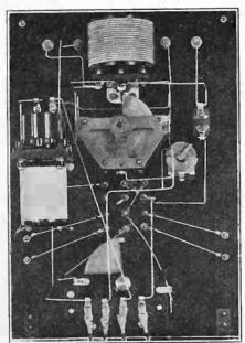
Inside View of Oscillator-Wavemeter.
