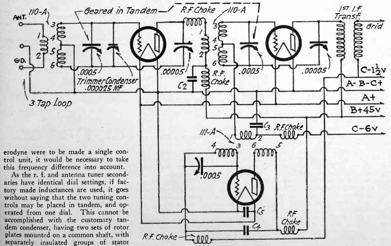
Fig. 1. Wiring Diagram for Tandem Control of Superheterodyne.
