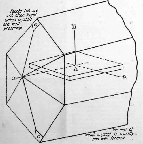
Fig. 2. Orientation of Axes in Quartz Crystal.
