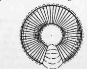
Fig. 3. Electromagnetic Field of Toroidal Coil.
