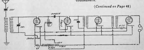
Fig. 1. Circuit for Tuned Plate Receiver.
