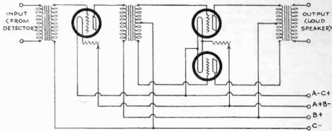
Fig. 10. Push-Pull A.F. Amplification.
