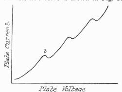
Fig. 3. Characteristic Curve of "Soft" Tube.
