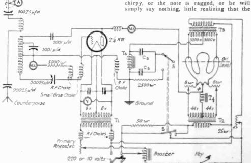
Fig. 2. Circuit Diagram for High Power Mercury Arc Transmitter,
