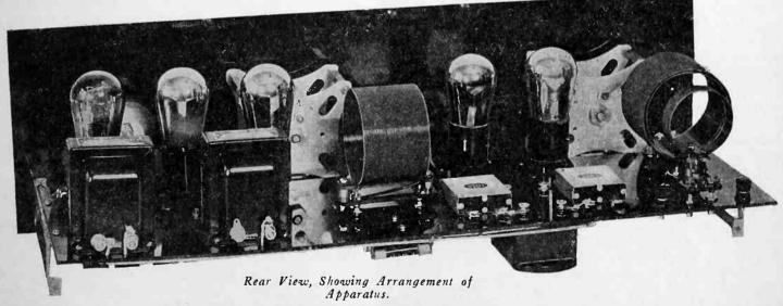
balancing condenser and the volume by a variable resistance in the audio amplifier, these adjustments having no effect on the settings of the tuning dials.
