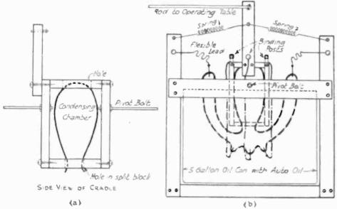
Fig. 1. A Simple Mercury Arc Shaker.
