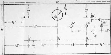
Fig. 2. Panel Layout for Shielded Superheterodyne.
