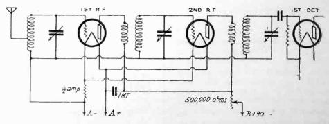
Fig. 3. New Plate and Filament Circuits for First Two Tubes.
