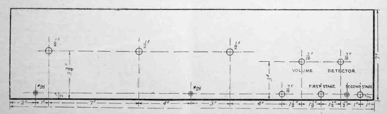
Fig. 3. Panel Drilling Template.
