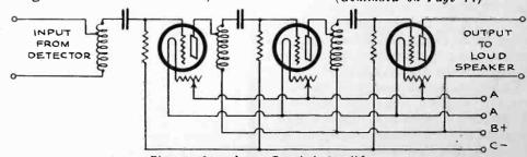
Fig. 12. Impedance Coupled Amplifier.
