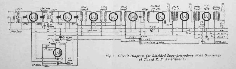
by hand if desired, so that the data for each coil are given in the following tables. The antenna tuner and r.f. transformer are identical, and consist of a stator form 2 in. wide by 21/2 in. long, with a rotor mounted inside the stator, made of a piece of bakelite tubing 1 in. wide and 3/4 in. long. Data are given for three different wavelength bands, so that any wave from 40 to 600 meters can be received.
