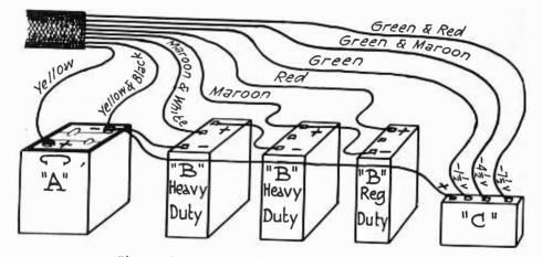
Fig. 3. Arrangement of Battery Cable Connections.
