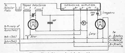
Fig. 1. Circuit Diagram for Infradyne Adapter.
