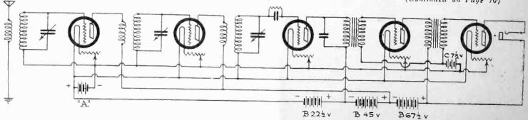
Fig. 6. Two Stages R.F., Detector and Two Stages A.F.
