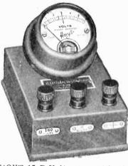
A HOYT 17-B Voltmeter, with high-resistance, moving-coil movement, and a hand-calibrated scale, 0-6 volts, marked in red at 3. Two tips are provided at the rear, for insertion in the panel tip-jacks, provided for the purpose in the R. C. A. Radiolas Nos. 20, 25, 26 and 28, and all the similar sets. the similar sets.
