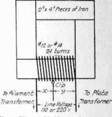
Fig. 3. Filament Line Booster for Steadiness.
