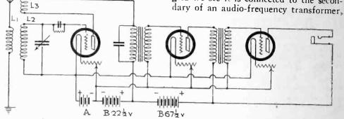
Fig. 5. Regenerative Circuit with Two Stages A.F. Amplification.
