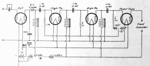
Fig. 2. Diagram of Impedance Coupled Amplifier Equipped with R. F. Choke.
