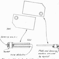
Fig. 4. Method of Adjusting Capacities.
