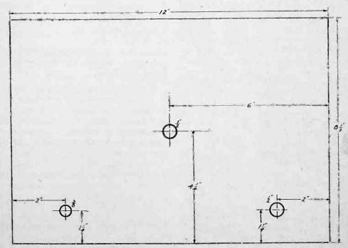
Fig. 4. Drilling Template for Panel and Shield.
