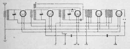
Fig. 1. Wiring Diagram of Crosley 5-38 Receiver.
