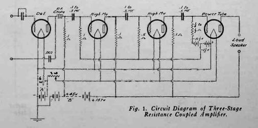
employed in the intermediate amplifier, if the set be a superheterodyne. If the condenser were made larger, it would present a fairly low resistance to the higher of the audio frequencies being amplified, and distortion would be introduced at an undesirable point in the circuit.
