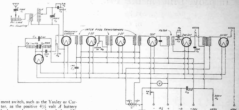
ter, as the positive  $4\frac{1}{2}$  volt A battery lead must be connected, and the additional pair of springs in the switch should be used to disconnect the power tube from the a.c. circuit. As the bell ringing transformer draws no current when the secondary load is removed, it may be left permanently across the a.c. line, and no switch in the primary is necessary or desirable.
