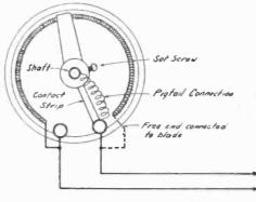
Fig. 2. Pigtail Connection for Rheostat.
