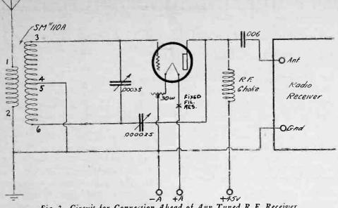
Fig. 3. Circuit for Connection Ahead of Any Tuned R.F. Receiver
