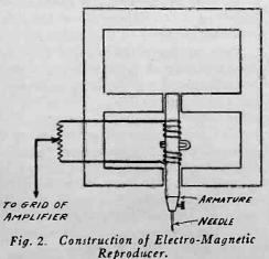
Fig. 2 shows the construction of the reproducer. The needle is solidly fixed in a small armature of soft iron. This armature is so regulated that it can move easily, following the wavy movement which is received from the needle which follows the lines of the disc. Around this armature is wound a solenoid coil of fine wire which is inserted in the strong magnetic field of a permanent magnet. The iron armature in vibrating back and forth inside this solenoid coil generates a feeble alternating
