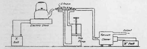
Fig. 1. Mechanical Illustration of Vacuum Tube Action.
