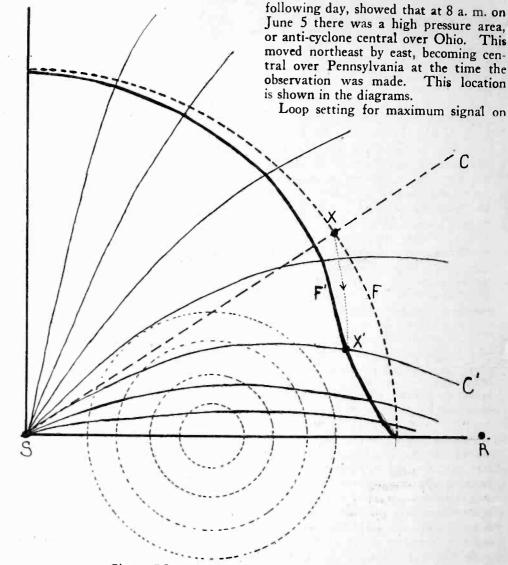
Fig. 5. Effect of Refracting Atmospheric Structures
