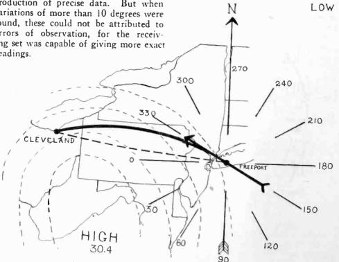
Fig. 4. Observed Deviation Due to High Pressure Area.
