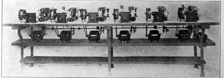
A Battery of Tungsten Filament Wire-Drawing Machines.
