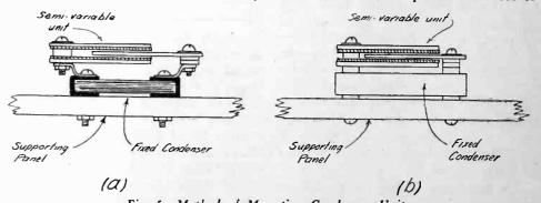
Fig. 5. Method of Mounting Condenser Units.
