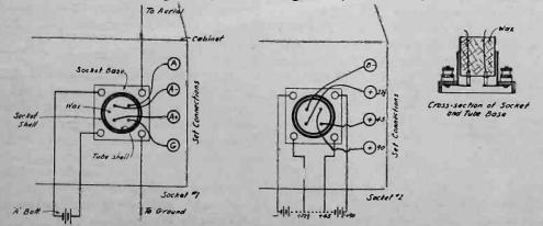
Fig. 1. Handy Antenna-Ground and Battery Connection,
