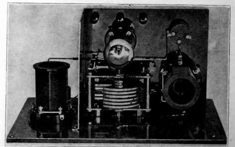
Amplifier Assembly, With Shield in Place.
