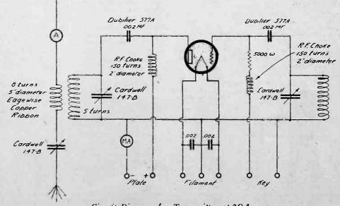
Circuit Diagram for Transmitter at 2QA.
