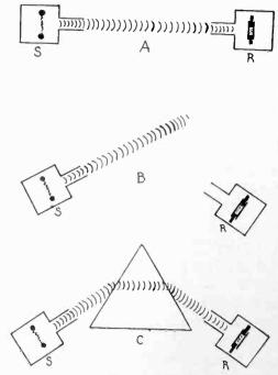
Fig. 1, Refraction of Radio Waves.
