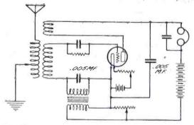
Fig. 2. Hookup Using One Tube as Detector A. F. and R. F. Amplifier.
