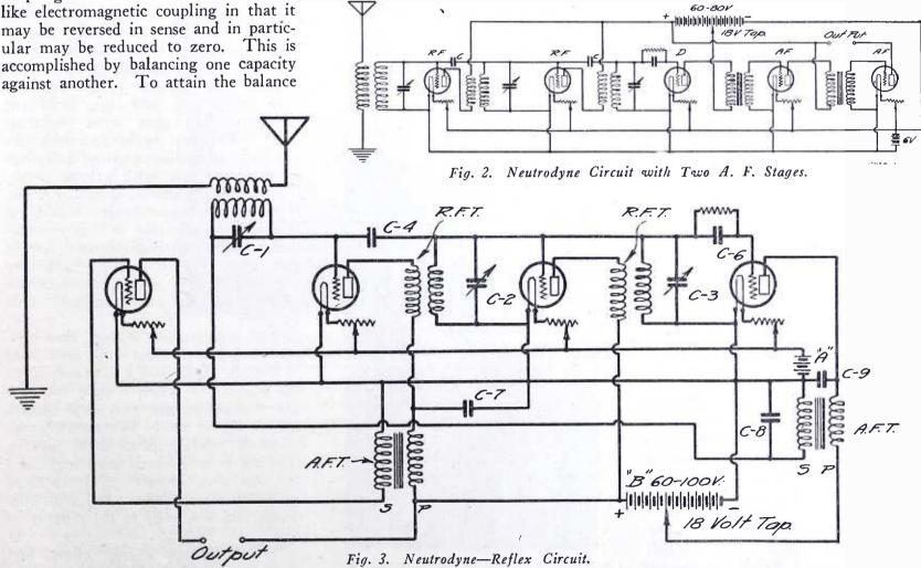
C<sub>4</sub>, C<sub>5</sub>—neutralizing condensers. C<sub>7</sub>, C<sub>8</sub>, C<sub>9</sub>—.001 mfd. fixed condensers.
