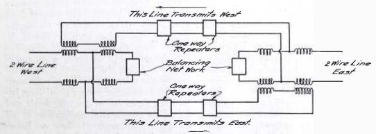
Fig. 3. Four-wire Line with One-way Repeaters.
