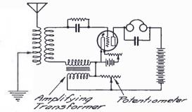
Fig. 1. Hookup for Audio Frequency Amplification.
