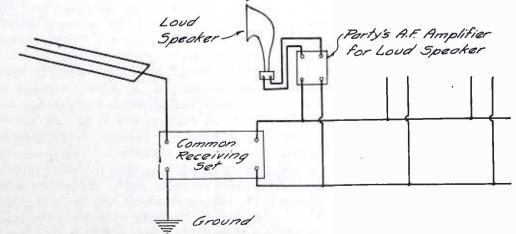
Plan 3. Common Antenna with Audio Frequency Distribution.
