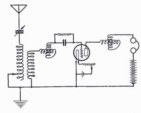
Fig. 4. Two Circuit Receiver Employing Plate Variometer Regeneration.
