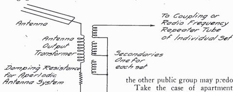
Plan 2. Common Antenna with Radio Frequency Distribution.
