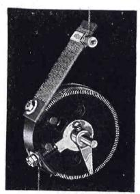
C-H Radio Resistance Unit Attached to Rheostat
