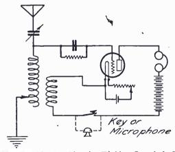
Fig. 5. Single Circuit Tickler-Coupled Set with Key or Microphone in Plate Lead.
