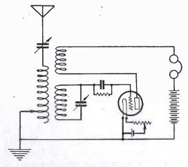
Fig. 3. Two Circuit Receiver Employing Tickler Regeneration.
