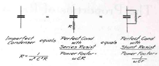
Fig. 1. Power Factors of Condensers
