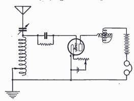
Fig. 2. Single Circuit Receiver Employing Plate Variometer Regeneration.
