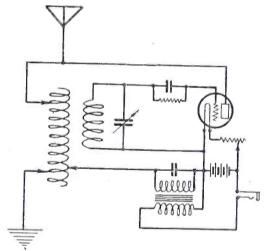
Fig. 1. Circuit Diagram for I. C. W. Transmitter
