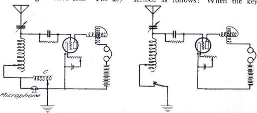
Fig. 7. Key or Microphone in Antenna Lead
