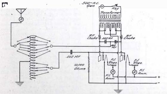
Fig. 1. Wiring Diagram of 1/2 K. W. Navy Spark Set Converted into 100 Watt Tube Set.
