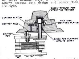
United Variable Condensers have a wonderful new patented Vernier Dial Control, which makes possible twice as fine adjustment as any three-plate Vernier on the market.
