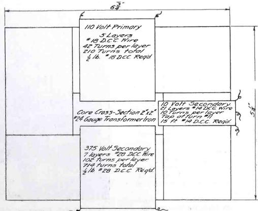
Fig. 2. Design for Power Transformer.
