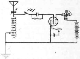
Fig. 8. Key in Grid Lead.
