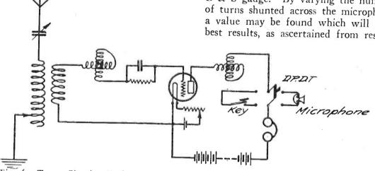
Fig. 6. Two Circuit Variometer-Coupled Set with Key and Microphone in Plate Lead.
