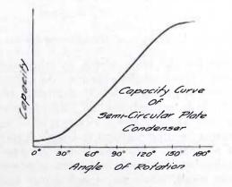
Fig. 3. Variation of Capacity with Rotation
