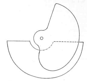
Fig. 6. Shape to Give Uniform Capacity
