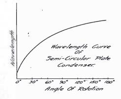
Fig. 4. Variation of Wavelength with Rotation
