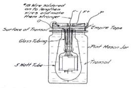
Fig. 1. Section showing 5-Watt Tube in Oil
