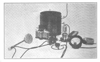
Fig. 25. View of 1/8 Watt Phone Circuit. This circuit utilizes a single receiving tube as an oscillator and can be operated entirely from five blocks of 22 wolt B batteries in series for the plate supply and a 6 wolt storage battery for heating the filament.
