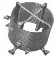
Standard size as shown consists of 25 turns of edgewise wound soft drawn copper ribbon 3/8 inch in width, 1/16 inch in thickness and the turns are SEVEN INCHES in diameter.
