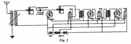
Question: I am sending you a drawing of my 50w C. W. set. I cannot get it to work. I have tested out all parts and found them working. When the tube is connected to the set, it doesn't light. Please tell me what is wrong.
