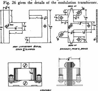
Fig. 26. Assembly of Modulation Transformer
