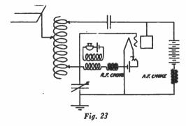
The antenna inductance as well as the plate coupling coil and grid input coil will be constructed as a single coil of 40 turns of No. 14 bare copper wire on a Bakelite or Micarta tube 5 in. in diameter and 6 in. in length. This tube should, preferably, have a 1/8 in. wall, though a thinner wall may be used with equal success if care is taken. The tube should be mounted in a lathe, and a spiral groove having a pitch of 1/8 in. should be cut to within  $\frac{1}{2}$  in. of each end.
