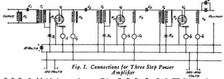
C<sub>1</sub> C<sub>2</sub> C<sub>6</sub> C<sub>4</sub>--2m.f.d. telephone condensers. Kellog Type 53 is suggested.
