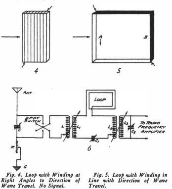
Fig. 6. "Antenna-Loop Barrage" Receiver
