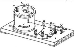
Fig. 6-Two-Circuit Tuner Connections
