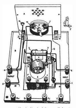
Fig. 1-Sketch of Detector Unit
