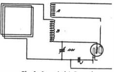
Fig. 2—Loop Aerial Connection
