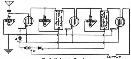
Fig. 3—Hook-up for Two Stages
