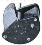
A quality product. Panel type. Plates of No. 20 heavy gauge aluminum. Plate separators gauged to ½ of 1-1000 of an inch, machine turned and nickel plated shaft. Top and base of ¼-inch sheet Bakelite Dilecto. Projecting shafts supplied on request.
