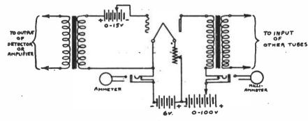
Fig. 1. Hook-Up for Testing Tubes
