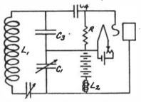
Fig. 6. Colpitts Laboratory Circuit.
