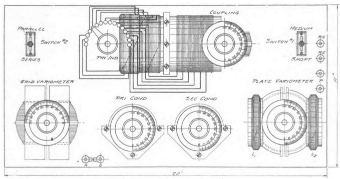
Fig. 2. Phantom View of Regenerative Receiver.
