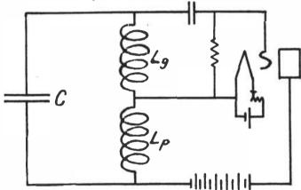
Fig. 4. Hartley Circuit as Used in the Laboratory.
