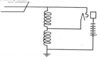
Fig. 1. The Hartley Circuit.
