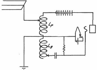
Fig. 5. Hartley Circuit as Used in Practice.
