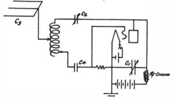
Fig. 7. Colpitts Circuit as Used for Transmission.
