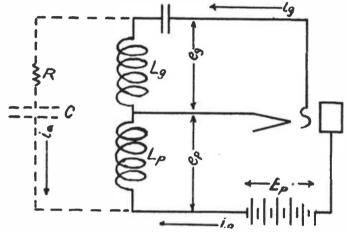
Fig. 2. Simplified Diagram of Hartley Circuit.
