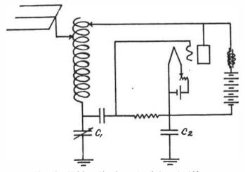
Fig. 10. Heising Circuit as Applied to the 938 set.
