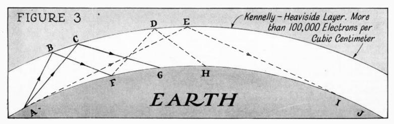
Based on the reflection theory the rays from the transmitter at point A are shown reflected downward by the radio roof and upward by the ground. The skipped distances are indicated.
