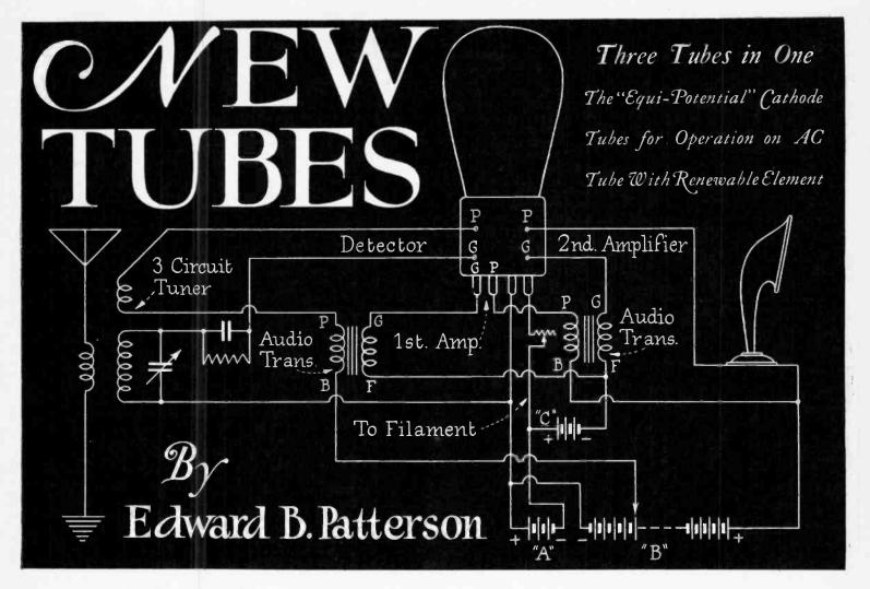
Figure 1. Ordinary three-circuit tuner hook-up adapted for the new three-in-one tube,
