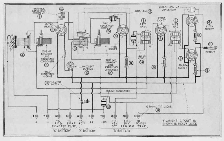
This diagram shows the wiring in the picture form.
