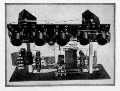
View looking from the rear showing receiver completely
