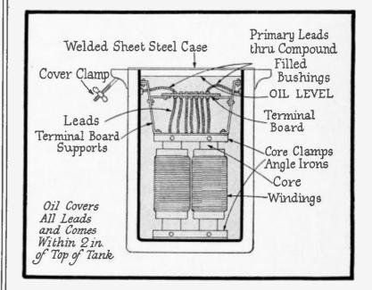
Above is a sectional view of the kind of power-line transformers blamed by most radio fans for interference. Mr. Allen's article explains its construction and shows that most of such complaints are not justified.
