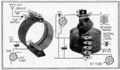
Showing correct connections to coils.
