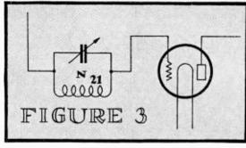
tem, such as a frame (loop acrial) and even allows the use of a special untuned aerial wire, without earth connection, as the sole stimulator. This diagram illustrates the 3electrode tube 16 used without H. F. (radio frequency) oscillation. Its grid and filament are joined across the circuit 17, which corresponds with the "N" in Figure 1. One point of this oscillator is joined to a point in the stimulating circuit.
