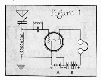
set can be rotated and meshed with a fixed set of plates without touching. Now, when two electrical conductors are placed in each other's vicinity, they have what is called a certain capacity, which means that a certain amount of energy can be "stored" in them, when one is charged positively, the other negatively. The capacity of two conductors then is dependent upon the total area and the distance between them, and also on the kind of material which separates them.
