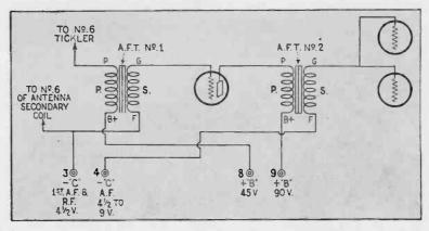
Completed sairing of the audio frequency amplifier circuit.
