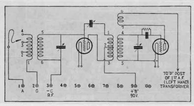
The wiring of the radio frequency and the detector circuits.
