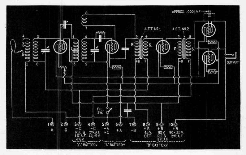
by tracing the path of the currents through the receiver. A stage of radio frequency amplification is used to increase the signal received in the antenna. This tube is neutralized to prevent radiation and annoying your neighbors.
