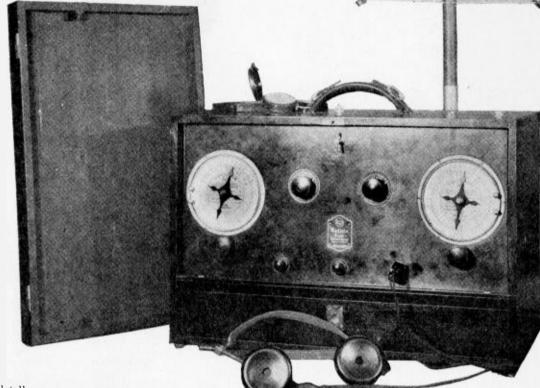
Here is the interference-hunting equipment used by one large power company. It is a super-heterodyne working on a directional loop.
