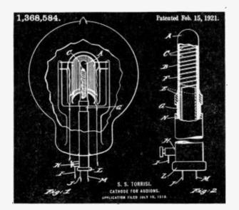
tungsten, the same as the filament and some difficulty was experienced in obtaining a copious supply of electrons because the construction did not permit the cathode to get as hot as the inside filament.
