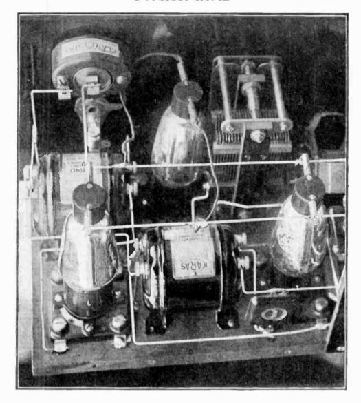
The heater connections are made with clips soldered to little wire springs which are, in turn, soldered to long pieces of hus wire. Note that the heater element connections come out at the top of the tubes.
