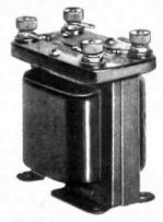
The finished job, of which we are mighty proud. The leads are soldered to tinned terminals, which are under nickel plated nuts over which are placed knurled nuts. Each binding post is plainly marked so that it is impossible to make incorrect connections.
