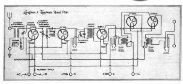
plate circuit of the radio frequency amplifying tube and really becomes a tuned circuit because it is so closely coupled to the variometer that the tuning of the variometer really tunes the plate circuit also.
