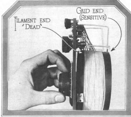
The coils are cor-rectly mounted when the end when the end which connects to the grid or grid condenser a re farthest from the panel. The effect of the hand is not exerted on the front end of the winding since it is at ground potential
