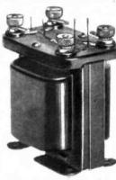
The wires extend through the Bakelite top, which affords perfect insulation, and are soldered to the terminals in plain sight, where they may be inspected. This also eliminates any possibility of breakage of transformer leads.
