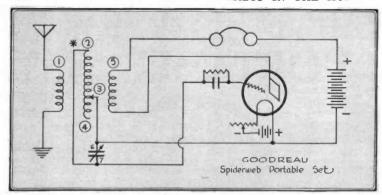
When using antenna or ground alone, connect at this point. When using both antenna and ground, connect as shown to primary coil
