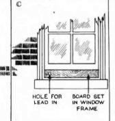
strand of wire so that the wire from C on down to the lightning switch is simply a continuation of the wire from B. In other words, you have one continuous wire beginning at the insulator B on the left. passing through the eyelet of C and on down to fasten to the insulator at E and then on down until it ends by being held fast under a screw head of the switch-blade at G. Both at C and at E it is merely passed through the eyelets of the insulators and is bound fast with
