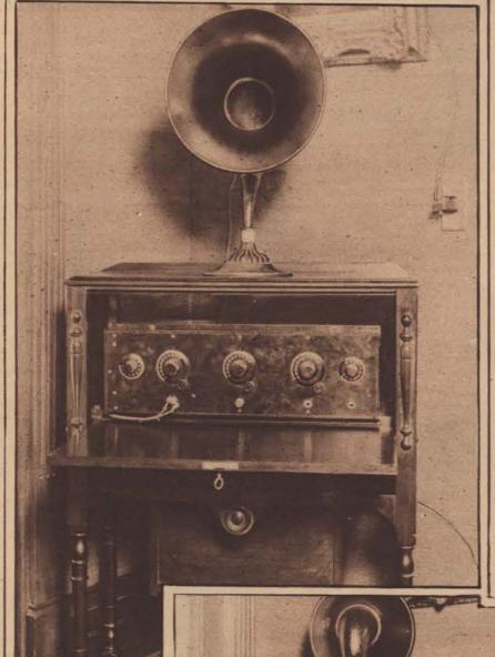
A typical neutrodyne installation with a Music Master horn, and a Ducon plug in the electric light socket for aerial and ground
