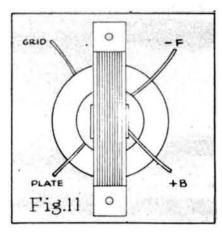
tion. It has been found, in fact, that the transformer with ratio of 1 to 4 or 5 generally gives greater step-up of voltage than one with a higher
