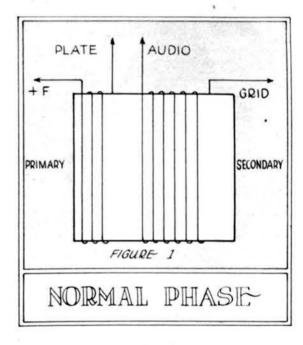
the two coils wound in the same direction of rotation, the above connections are called "normal phase." To connect the secondary in "reverse phase," merely means to connect the grid to the end nearest the primary. Figure 2 shows the coil with this reversal. This reversal, together with the proper alignment of the tuned coils, eliminated the radio oscillation.
