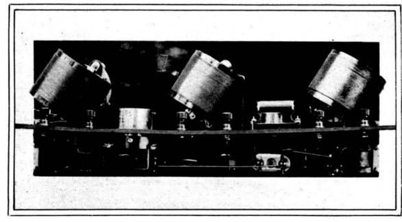
A view from the back showing the angle of the neutroformers could be overcome by slightly detuning the condenser in the crystal circuit. There was found to be no need for the neutrodons or neutralizing condensers as employed in the Hazeltine circuit, and so they were not connected. A further investigation of this showed that the neutroformers used had only six turns on the primary windings. Perhaps this explains their lack of oscillation even without the neutrodons. were made by Fada.
