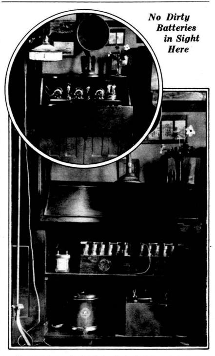
These two photographs show the installation in the home of H. W. Leeds, 107 North Thirty-fourth Street, Philadelphia, Pa. The bottom compartment of the desk contains storage, A, B and C batteries with chargers and with the switching arrangement given not long ago in RADIO IN THE HOME. It is only necessary to throw a switch from "use" to "charge" to freshen up any of the batteries for further use.
