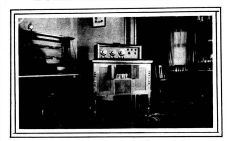
Here is a clever installation in the home of Dr. J. H. Rice, of 718 West French Place, San Antonio, Texas. The cabinet is mounted upon ball-bearing felt rollers so that it can be moved from one room to another and in all rooms there are bakelite connections on the walls for jacks and plugs for antenna and ground. The cabinet contains all batteries and a full-sized loud speaker. This is the kind of installation that is going to help spread radio.
