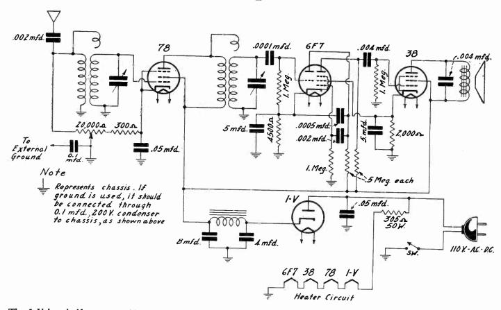
The 1-V is a half-wave rectifier, useful in universal sets particularly, especially when the current drain is not high enough to warrant the use of the 25Z5, although even that is not to be considered a high current type rectifier by any means. The circuit is one of the simplest four tube t.r.f. midgets.
