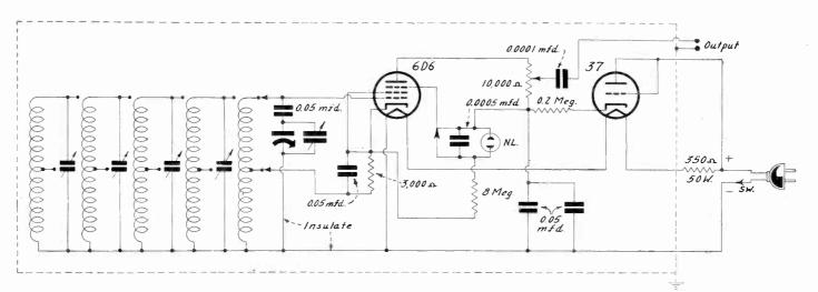
A signal generator with rectifier.
