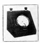
Meters are put in cases as shown, for convenience and protection. This meter is of the single range variety.
