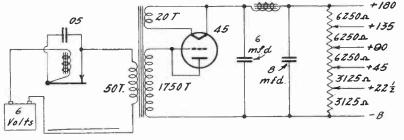
Even with a vibrator is used the voltages taken off may be anything from maximum to intermediate values, by the voltage divider method as applied to other rectifier systems. An example is cited at right.
