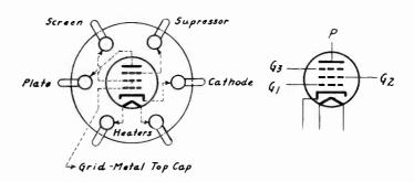
The socket connections for the 57 or 6C6 are shown at left. The elements are (bottom view) identified in connection with standard numerical location of base pins. At right the elements are identified, also the grids in terms of numerical order, i.e., grid No. 1 is control grid, No. 2 is screen and No. 3 is plate.
