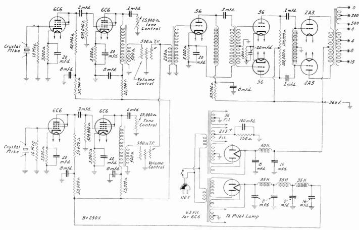
The 750 ohm power tube biasing resistor has 100 mfd. across it.
