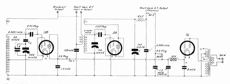
The triode is used as a rectifier sometimes, when the current drain is even smaller than that considered above. Thus, in the diagram above, two 58 tubes are served by a 76 used as diode, with grid tied to plate, the preferable way for a.c. line rectification, because of the limited capabilities of grid alone as to current. A broadcast oscillator at left, with short wave set in center for reception or transmission.
