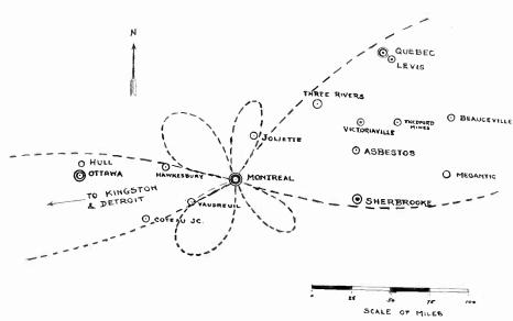
The directive array servicing the Quebec section (right) has been designed to be broad, as 200-mile coverage is all that need be expected, while the beam towards Ottawa (left) has been made for as high a power gain as possible, so that long distances to Toronto, Windsor, Detroit and Chicago eventually can be covered.
