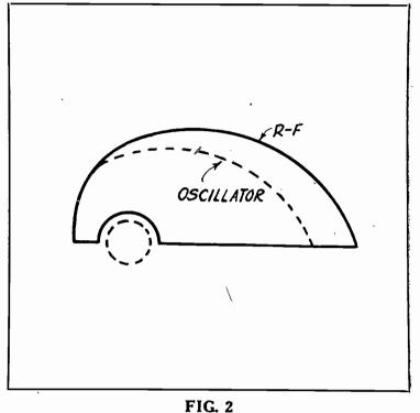
This illustrates how the plates of a tracking condenser are shaped to produce tracking. The oscillator condenser plates are smaller as shown by the dotted line.
