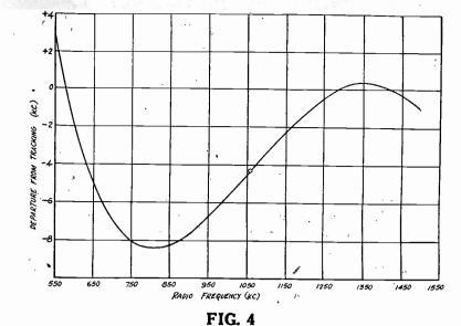
A typical tracking curve obtained by the padding method as exemplified in Case I. The tracking indicates excessive oscillator inductance.
