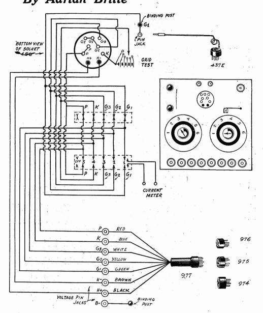
not be put into the universal socket, so an adapter is used that permits testing when a seven-pin tube is met. The seven-pin tube is finally released now by the licensed group of tube manufac-turers as a whole, it being the 59 power tube, which, by various grid interconnec-tions, may be a Class A amplifier (pen-tode or triode type), or a Class B output tube. With Class B two tubes must be used in the output in push-pull form. (Continued on next page)
