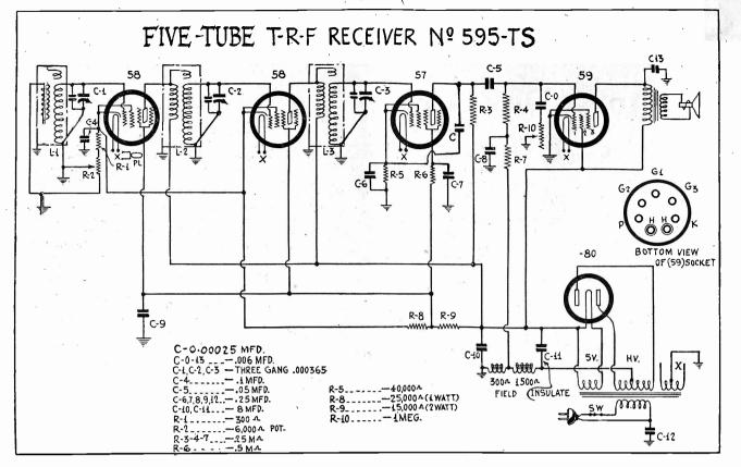
7 per cent. is 8.4 per cent. The way to keep the distortion in the 59 to as low a figure as in the other instance, and at the same time to increase the power output as well, is to use a 6,000 ohm load. The result is 7 per cent. total distortion (as with the '47) but a power output at that distortion' level of 3 watts, compared to 2.5 watts for the '47.
