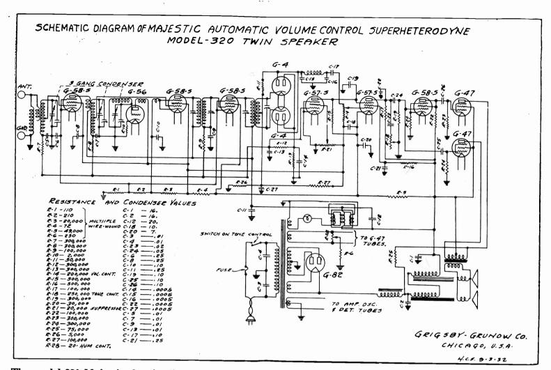
The model 320 Majestic chassis, diagram above, is used in the model 324 receivers. Model 320 circuit is identical with model 300 circuit except that 324 has delayed a-v-c.
