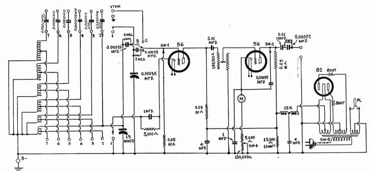
Three-tube modulated oscillator (with switch SW-1 for modulation removal), 170 to 60,000 kc, with converter and vacuum tube voltmeter built in.
