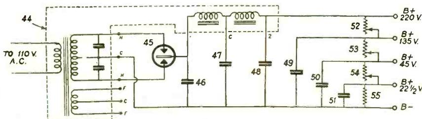
THE B POWER SUPPLY USES A RAYTHEON TUBE AND A THORDARSON COMPACT. THIS PARTICULAR UNIT IS EXTREMELY SIMPLE TO ASSEMBLE AND WIRE, AND GIVES ALL-SUFFICIENT VOLTAGE EVEN AT HIGH CURRENT DRAIN.
