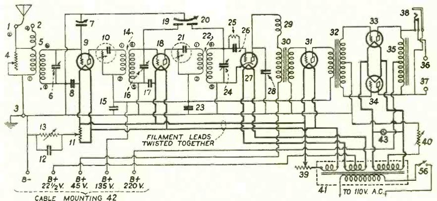
PICTORIAL DIAGRAM OF THE WIRING OF THE RECEIVER. FINE SENSITIVITY, WITHOUT APPRECIABLE HUM, IS ATTAINED IN THE SUPREME AC SIX, WHICH HAS AS ITS FINAL AUDIO STAGE A PUSH-PULL CIRCUIT, WHICH DOES MUCH TO RID THE CIRCUIT OF HUM, BESIDES KEEPING THE TONE QUALITY LEVEL HIGH. PUSH-PULL TENDS TO SUPPRESS THE EVEN HARMONICS, AND AS THE SECOND HARMONIC IS THE MOST PROFUSE SOURCE OF TUBE DISTORTION, THE QUALITY IS SPLENDID ALTHOUGH THE IMPRESSED SIGNAL VOLTAGE MAY BE HIGH.
