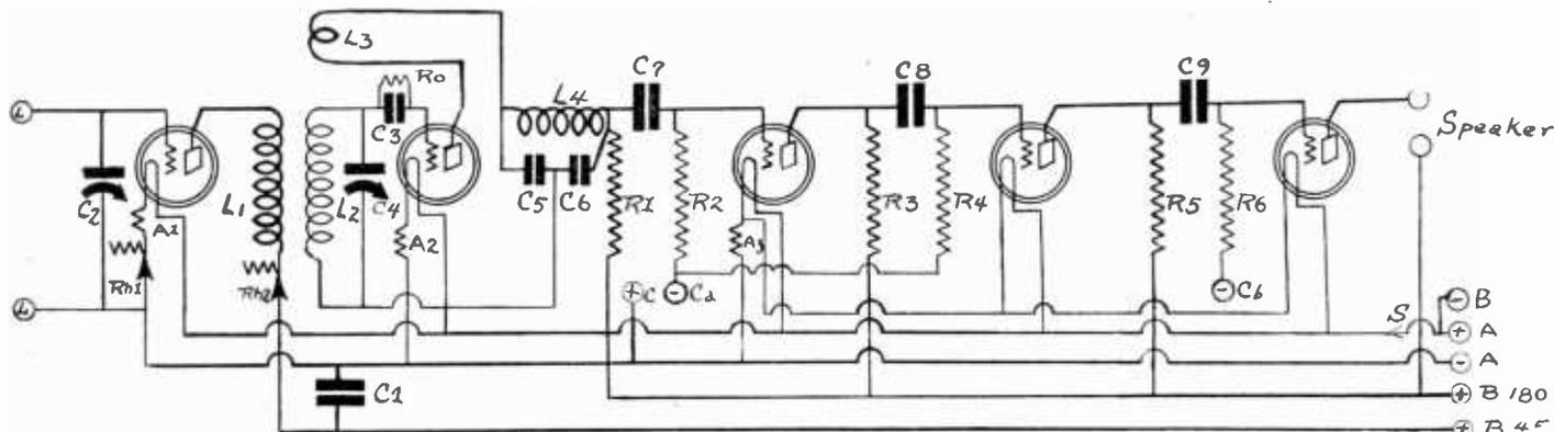
THE circuit diagram of the high quality receiver described by Tim Turkey. Even amplification from the lowest audible to the highest essential frequency is a feature of this receiver. Additional directions for building and operating the receiver are given in the present issue. Freedom from motorboating was emphasized in designing the set.
