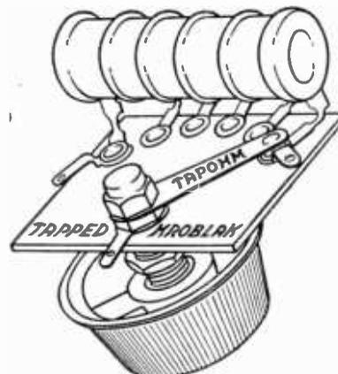
The latest addition to the line of Mountford resistances and Kroblaks is the Kroblak variable resistor of approximately 30,000 ohms, tapped in five equal sections. This unit makes an excellent output control device for B eliminators. The total capacity is 10 watts and the overall size is 2x2x2 1/4 inches. This unit is made by C. E. Mountford, Sullivan Street, New York City.
