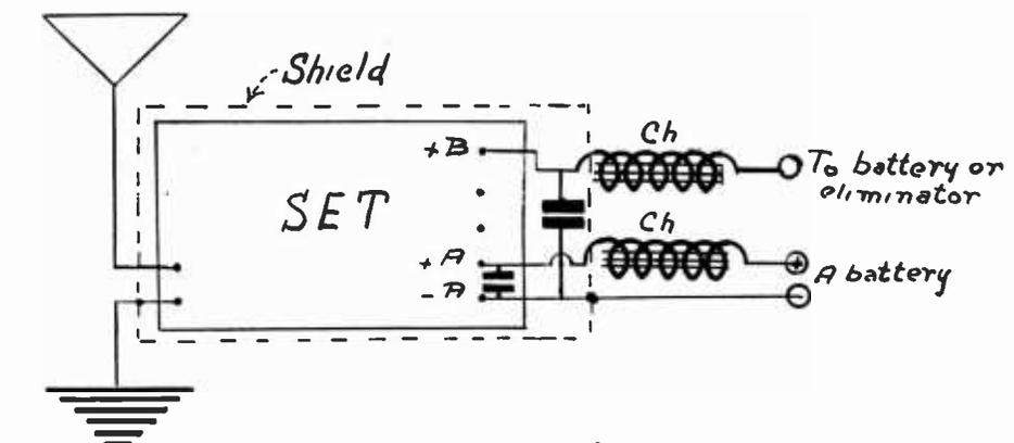
HOW the receiver should be shielded and how choke coils and by-pass condensers should be placed when unshielded batteries or eliminators are used, or when the leads to power source are long.
