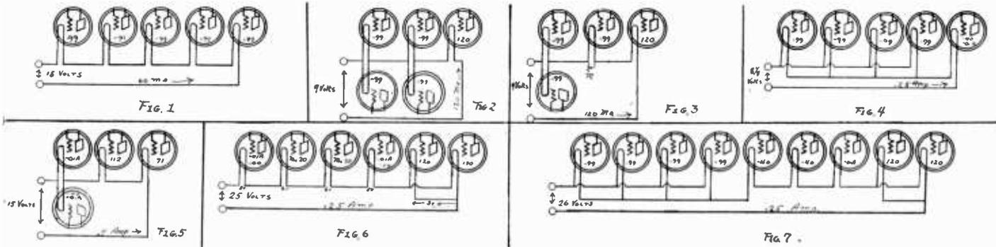
RECEIVERS in which the filaments are connected in series are gaining in popularity. The reason for this is the desire to eliminate all batteries from the receivers.
